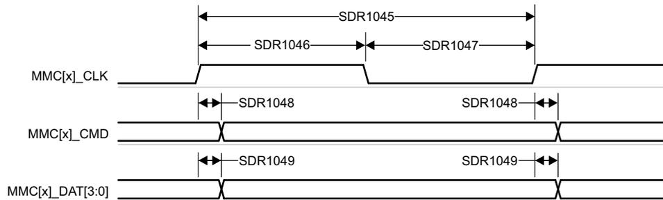
**Figure 6-95. MMC1/MMC2 – UHS-I SDR104 – Transmit Mode**
