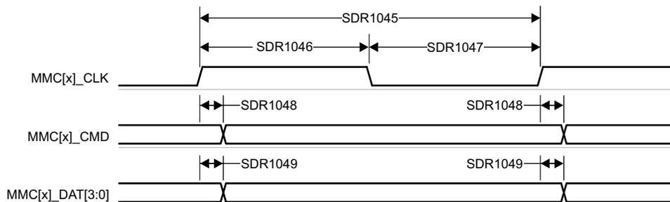
**Figure 6-84. MMC0 – UHS-I SDR104 – Transmit Mode**
