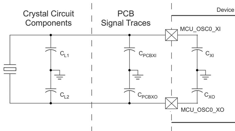
**Figure 6-18. Load Capacitance**
