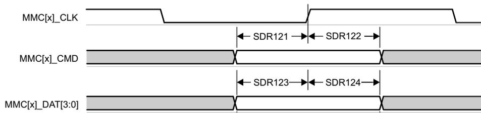
**Figure 6-89. MMC1/MMC2 – UHS-I SDR12 – Receive Mode**
