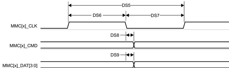
Figure 6-75. MMC0 – Default Speed – Transmit Mode
