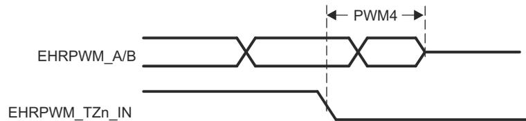
**Figure 6-44. EHRPWM\_TZn\_IN to EHRPWM\_A/B Hi-Z Switching Characteristics**
