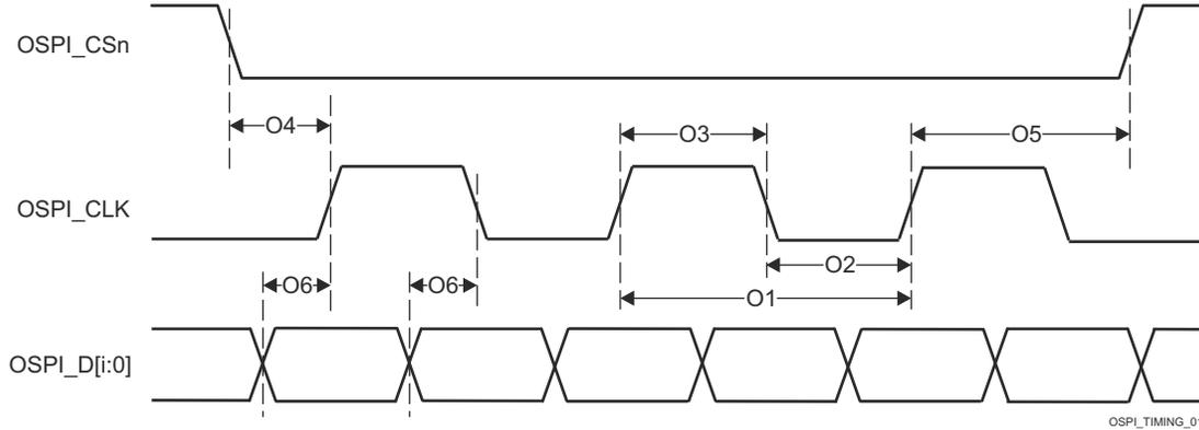
**Figure 6-108. OSPI0 Switching Characteristics – Tap DDR, No Loopback**
