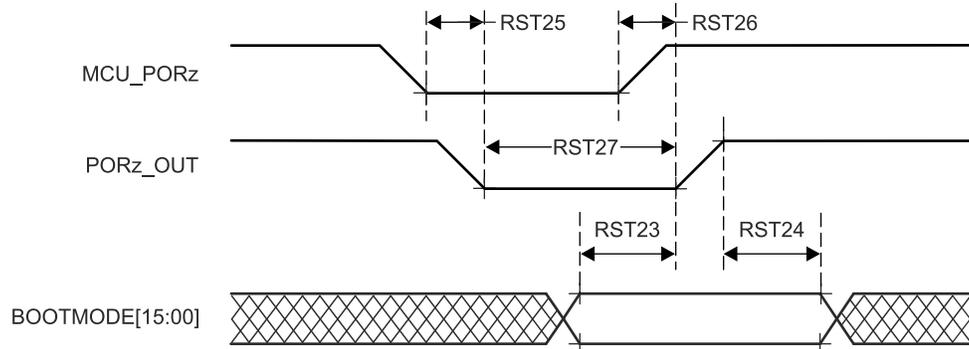
**Figure 6-12. BOOTMODE Timing Requirements and PORz\_OUT Switching Characteristics**
