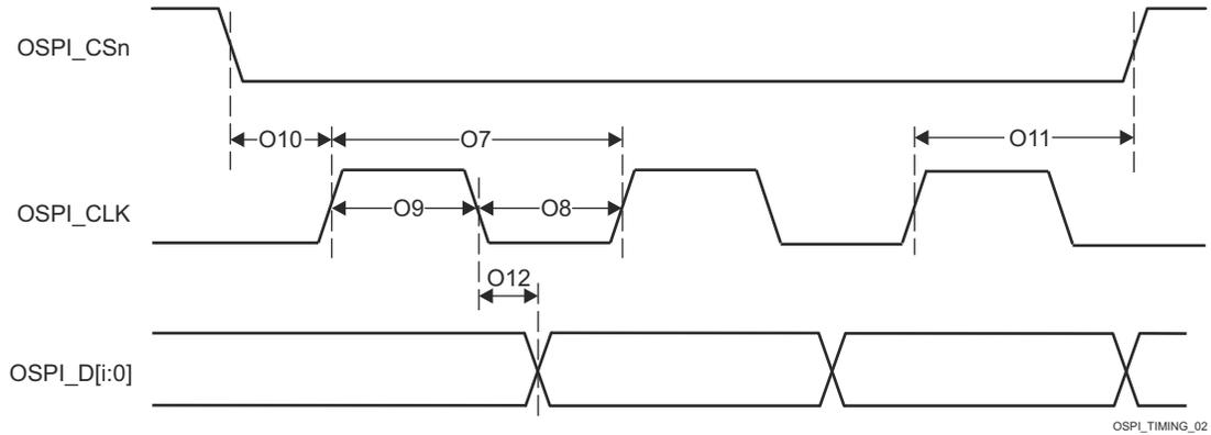
**Figure 6-99. OSPI0 Switching Characteristics – PHY SDR Data Training**
