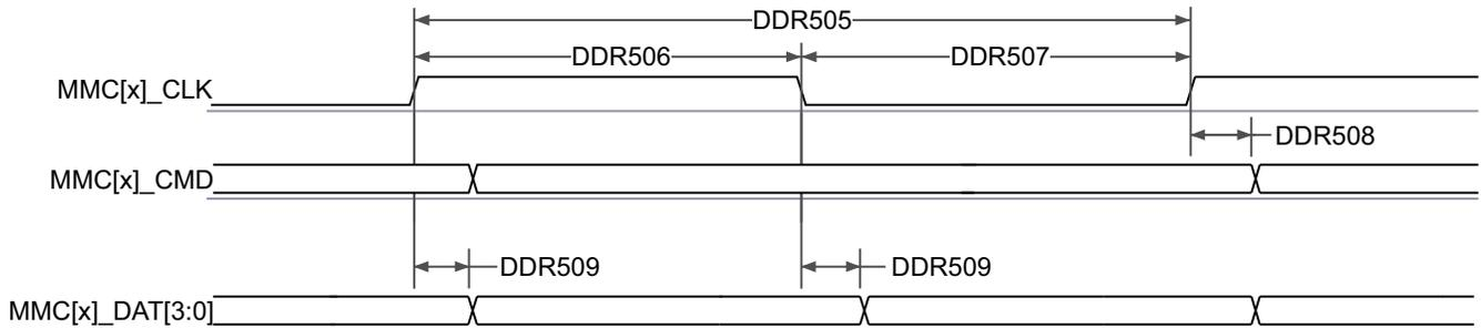
**Figure 6-94. MMC1/MMC2 – UHS-I DDR50 – Transmit Mode**
