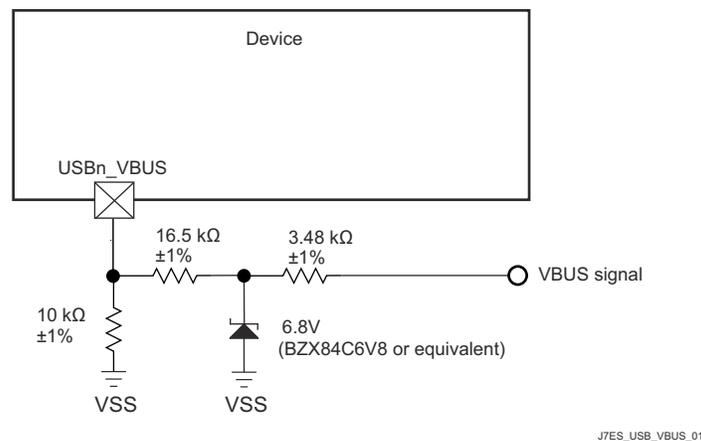
**Figure 8-4. USB VBUS Detect Voltage Divider / Clamp Circuit**
