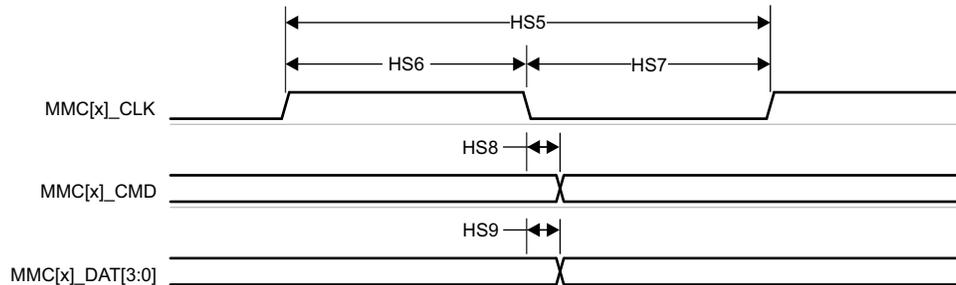
**Figure 6-77. MMC0 – High Speed – Transmit Mode**
