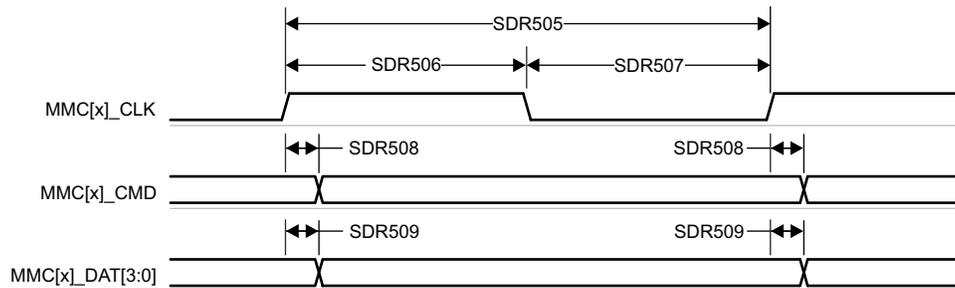
**Figure 6-93. MMC1/MMC2 – UHS-I SDR50 – Transmit Mode**
