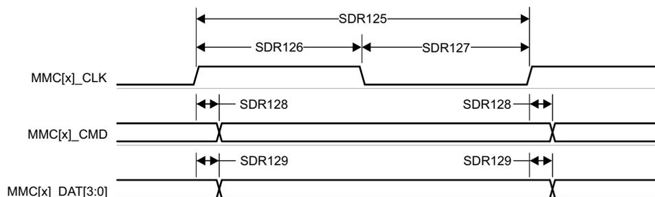
**Figure 6-90. MMC1/MMC2 – UHS-I SDR12 – Transmit Mode**
