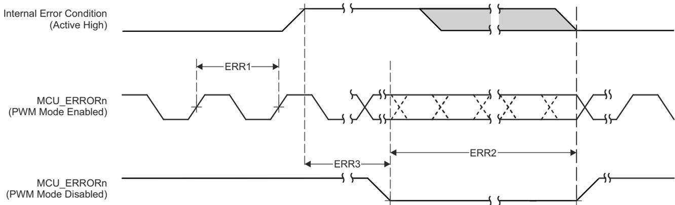
**Figure 6-13. MCU\_ERRORn Timing Requirements and Switching Characteristics**
