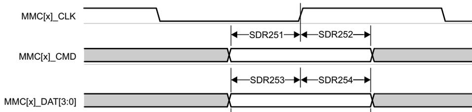
**Figure 6-91. MMC1/MMC2 – UHS-I SDR25 – Receive Mode**
