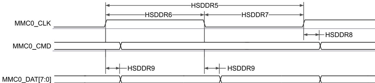
Figure 6-72. MMC0 – High Speed DDR Mode – Transmit Mode
