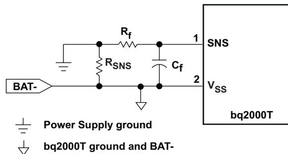
**Figure 8. Current-Sensing Circuit**
