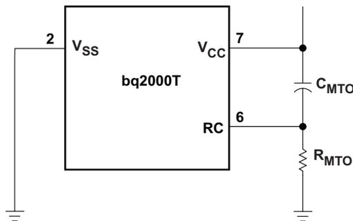
Figure 5. Typical Connection for the RC Input
