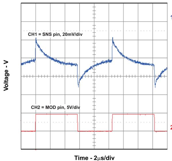
Figure 17. bq2000T Fast Charge SNS and MOD Waveforms
