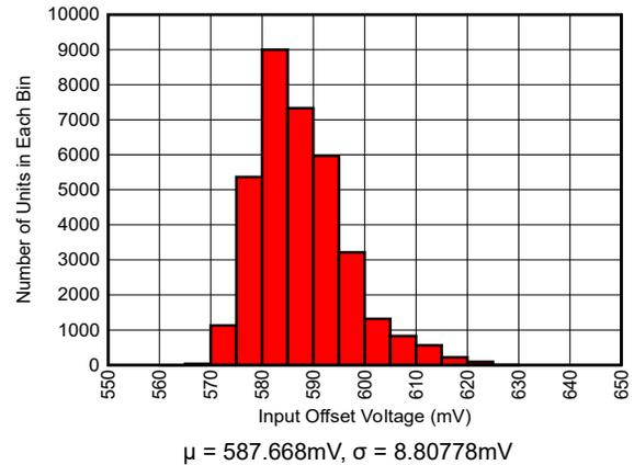
Figure 5-30. Offset Voltage Histogram
