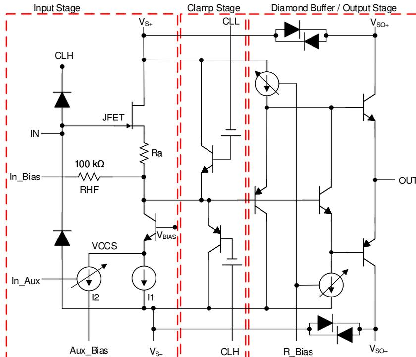
The functional block diagram shows an overview of the internal structure of the BUF802. The internal schematic of the BUF802 is divided into the following three parts:
