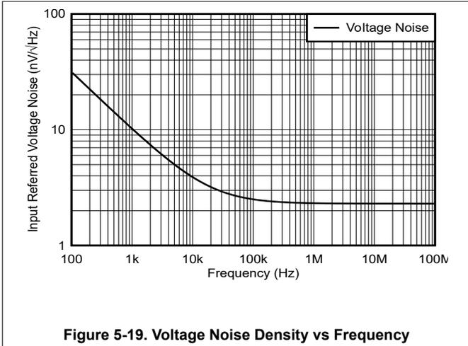
**Figure 5-19. Voltage Noise Density vs Frequency**
