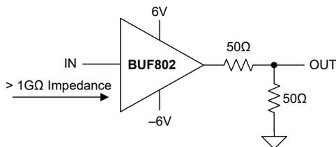
Impedance Transformation Circuit Using the BUF802
