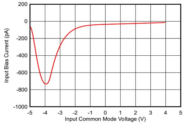
Figure 5-26. Input Bias Current vs Input Common-Mode Voltage
