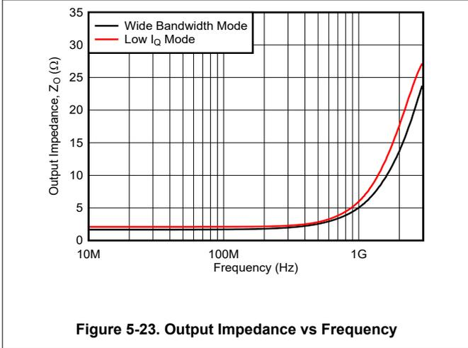
**Figure 5-23. Output Impedance vs Frequency**
