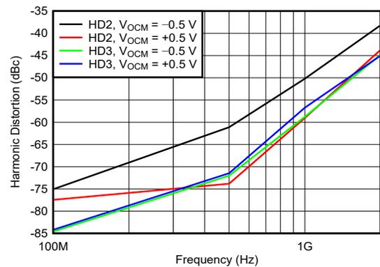
Figure 5-16. Harmonic Distortion vs Output Common-Mode Voltage
