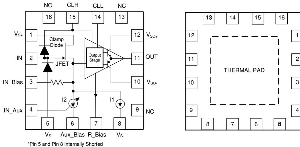
**Figure 4-1. RGT Package, 16-Pin VQFN
