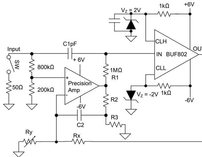
Figure 7-13. Composite Loop Using *BF Mode*
