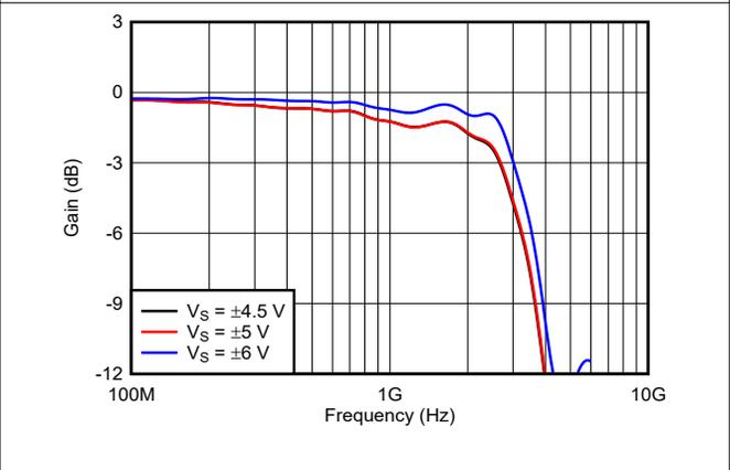
Figure 5-4. Frequency Response vs Supply Voltage
