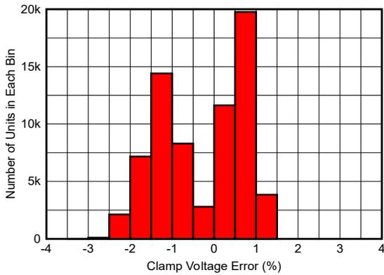
**Figure 5-33. Clamp Voltage Error Histogram**
