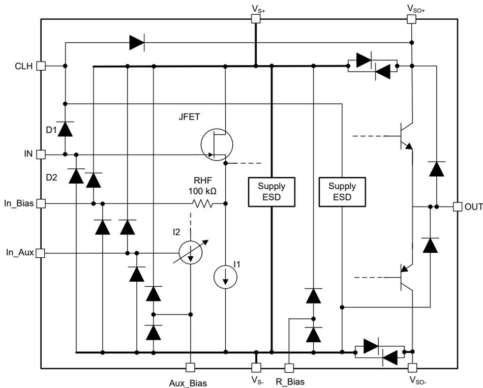
Figure 7-7. Internal ESD Structure
