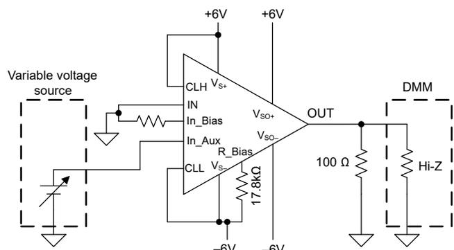
**Figure 6-3. Auxiliary Path Electrical Characteristics Measurement**
