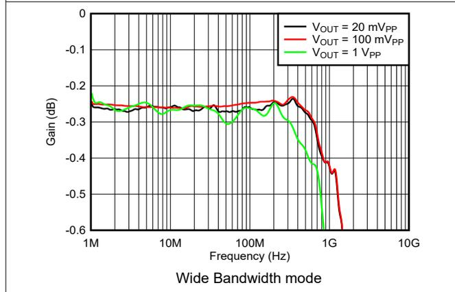
Figure 5-3. Frequency Response vs Output Voltage, 0.1dB Flatness
