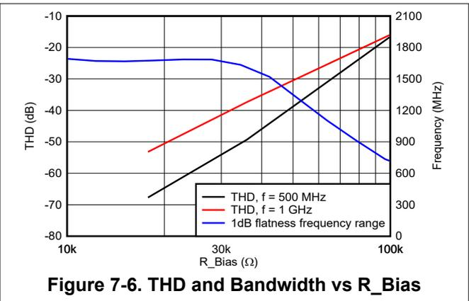
The [Figure 7-6](#) shows that changing the resistor between the  $R_{Bias}$  and  $V_{S-}$  primarily affects the THD of the output signal. [Section 5.5](#) and [Section 5.6](#) specify the AC and DC parameters of the BUF802 at two different  $R_{Bias}$  values. The DC parameters are independent of the quiescent current setting.
