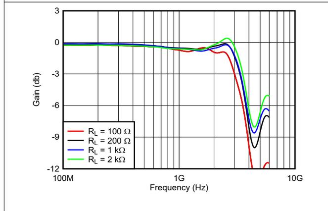
Figure 5-5. Frequency Response vs Output Load
