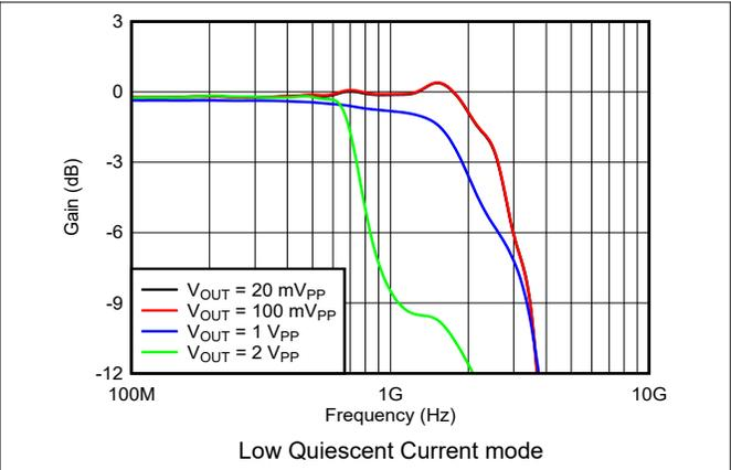
Figure 5-2. Frequency Response vs Output Voltage
