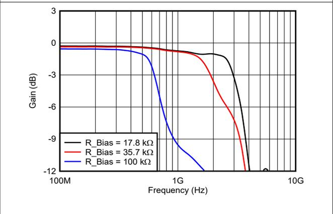
Figure 5-6. Frequency Response vs  $R_{\text{Bias}}$  Resistance
