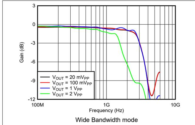
Figure 5-1. Frequency Response vs Output Voltage
