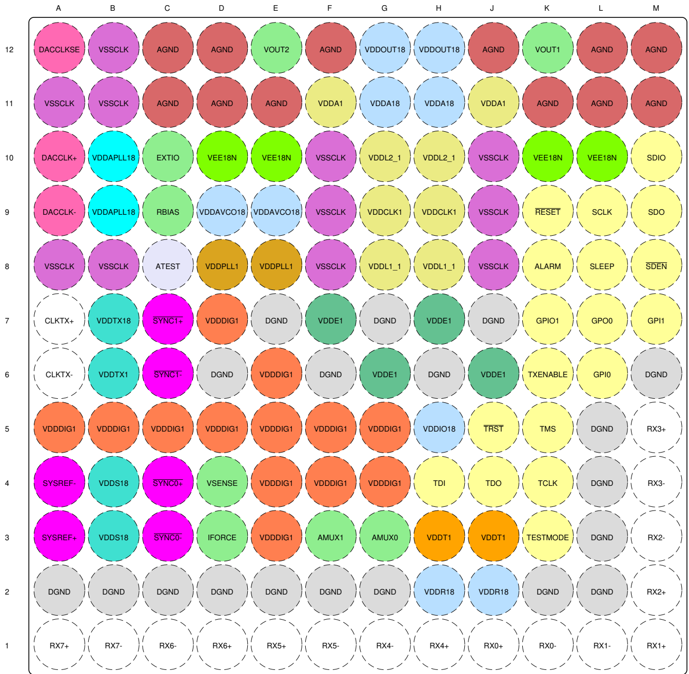
Figure 5-2. DAC38RF80, DAC38RF84, DAC38RF90 AAV Package 144-Pin (FCBGA) 144-Pin FCBGA Top View
