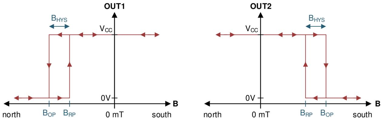
**Figure 7-4. Unipolar Functionality**
