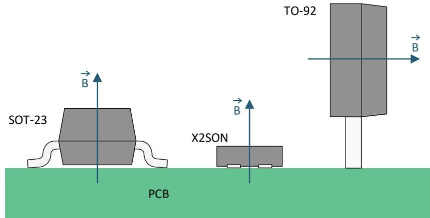
**Figure 7-1. Direction of Sensitivity**
