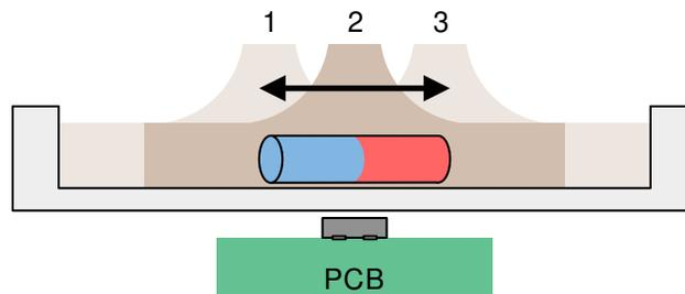
Figure 8-4. Three-Position Slider Switch With Embedded Magnet
