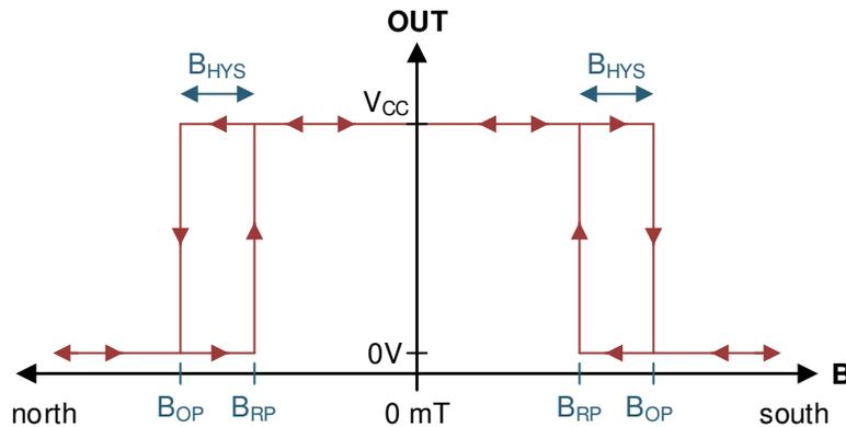
**Figure 7-3. Omnipolar Functionality**
