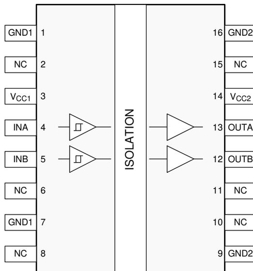
**Figure 5-1. ISO7720 DW Package 16-Pin SOIC Top View**
