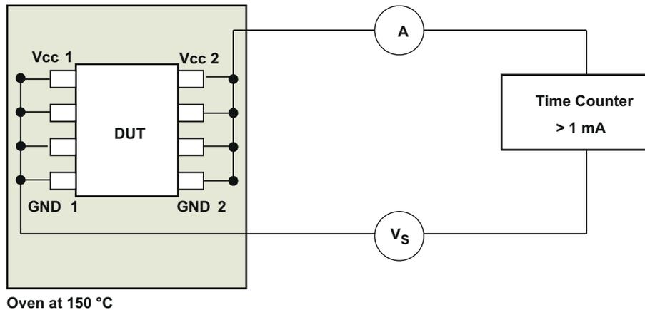
**Figure 9-5. Test Setup for Insulation Lifetime Measurement**
