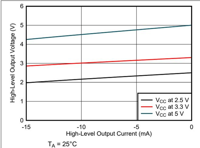
Figure 6-11. High-Level Output Voltage vs High-level Output Current
