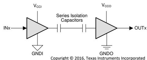
V<sub>CCI</sub>=Input supply, V<sub>CCO</sub>=Output supply
