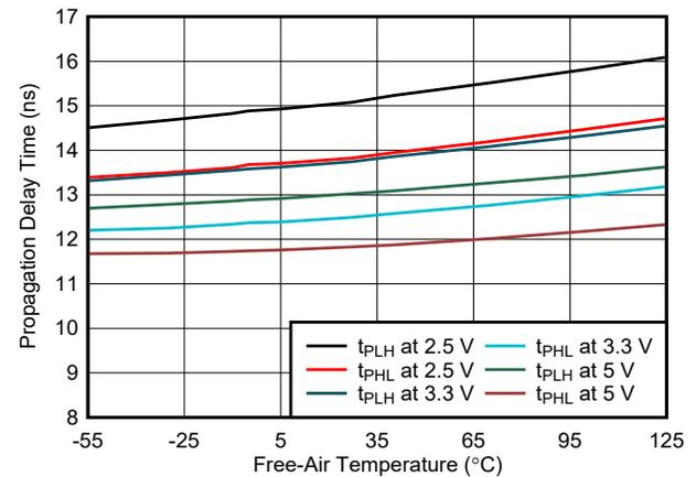
Figure 6-14. Propagation Delay Time vs Free-Air Temperature
