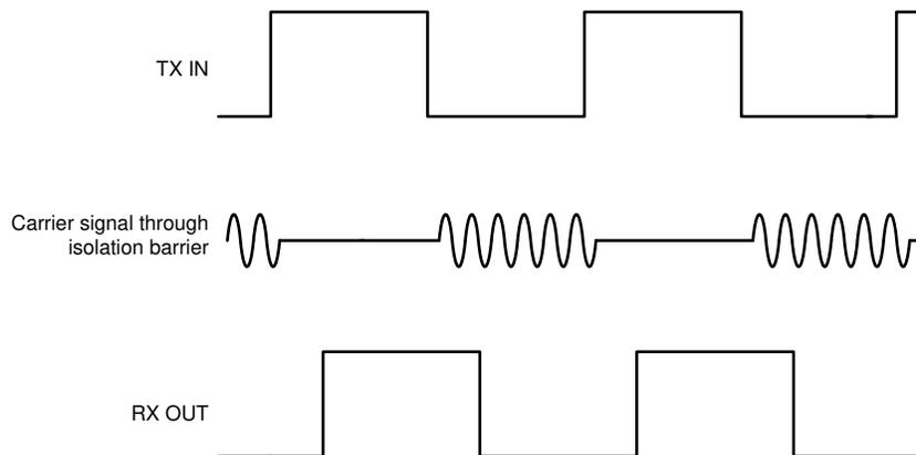
**Figure 8-2. On-Off Keying (OOK) Based Modulation Scheme**
