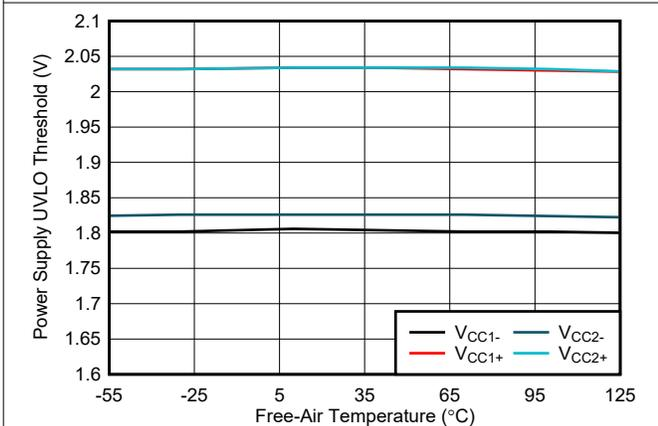
Figure 6-13. Power Supply Undervoltage Threshold vs Free-Air Temperature
