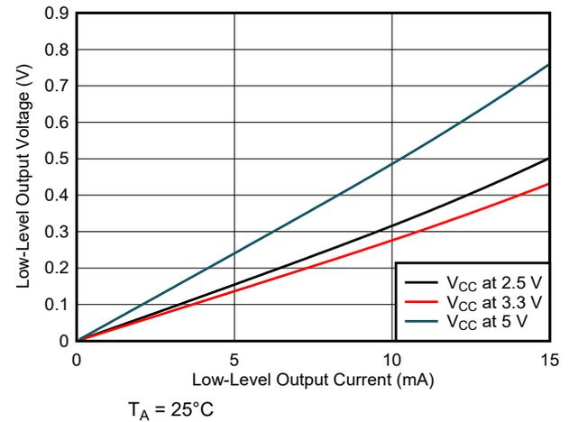
Figure 6-12. Low-Level Output Voltage vs Low-Level Output Current
