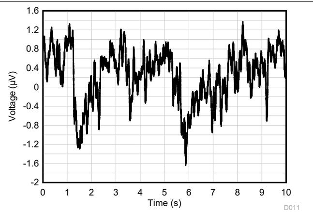
Figure 5-16. 0.1-Hz to 10-Hz Noise
