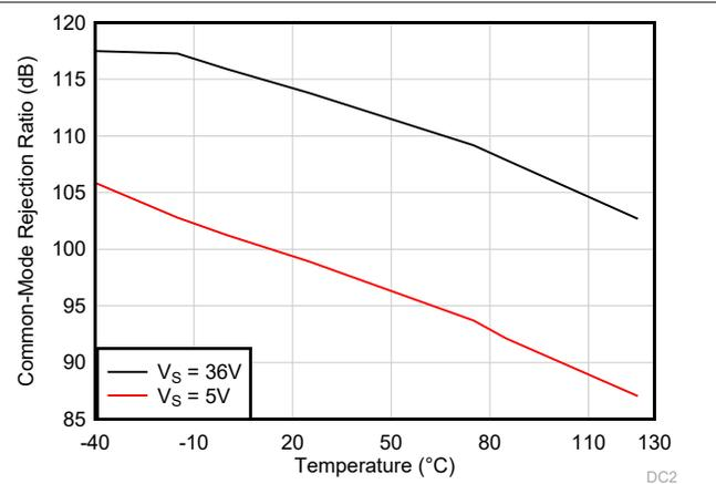
Figure 5-14. Common-Mode Rejection Ratio vs Temperature (dB)
