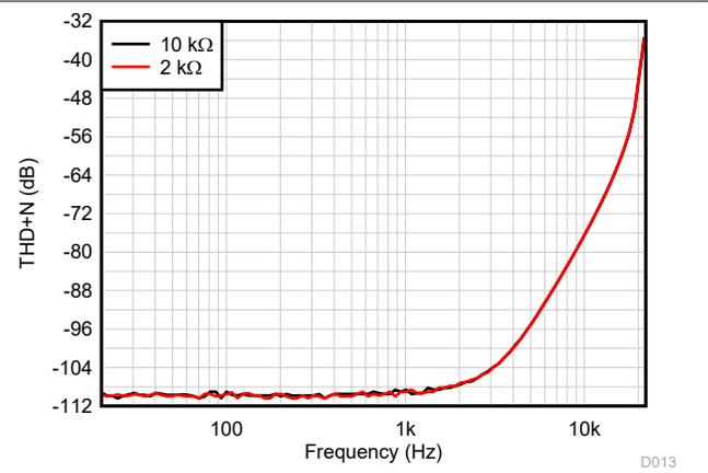
Figure 5-18. THD+N Ratio vs Frequency,  $G = 1$
