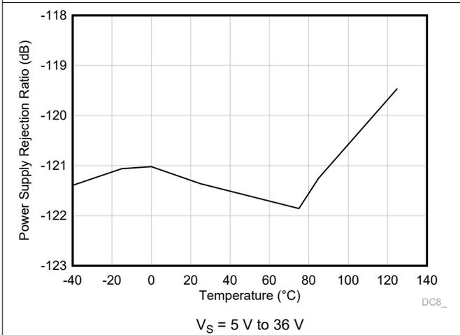
Figure 5-15. Power Supply Rejection Ratio vs Temperature (dB)
