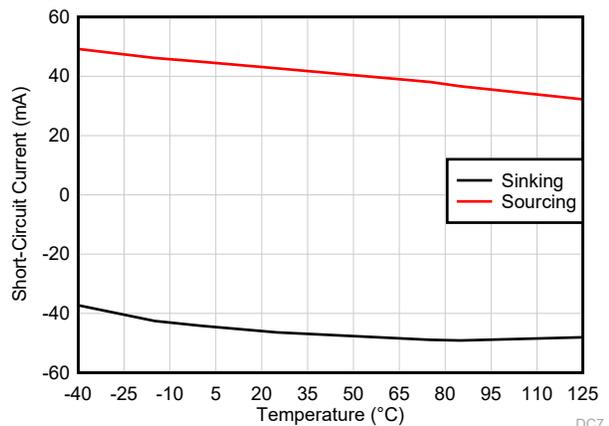
Figure 5-35. Short-Circuit Current vs Temperature
