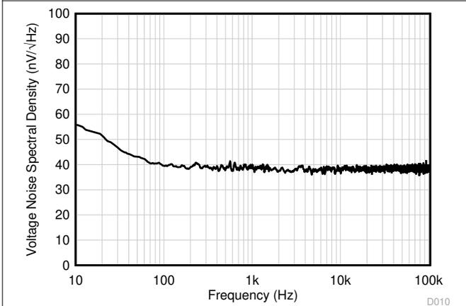
Figure 5-17. Input Voltage Noise Spectral Density vs Frequency
