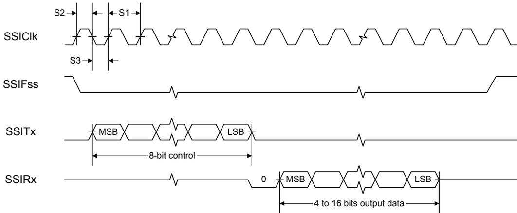
Figure 19-13. SSI Timing for SPI Frame Format (FRF=00), with SPH=1
