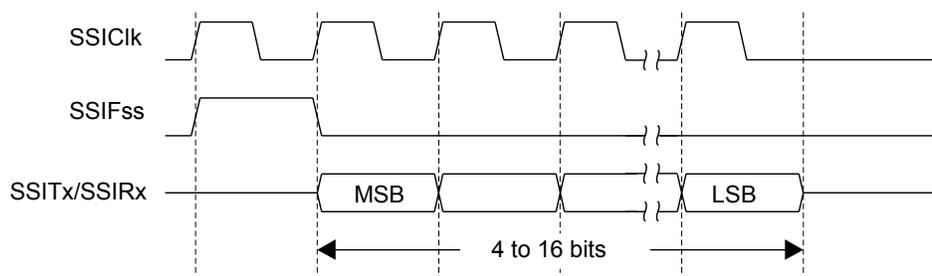
In this mode,  $SSIClk$  and  $SSIFss$  are forced Low, and the transmit data line  $SSITx$  is tristated whenever the SSI is idle. Once the bottom entry of the transmit FIFO contains data,  $SSIFss$  is
