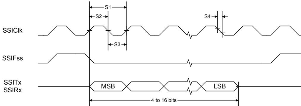
**Figure 19-12. SSI Timing for MICROWIRE Frame Format (FRF=10), Single Transfer**
