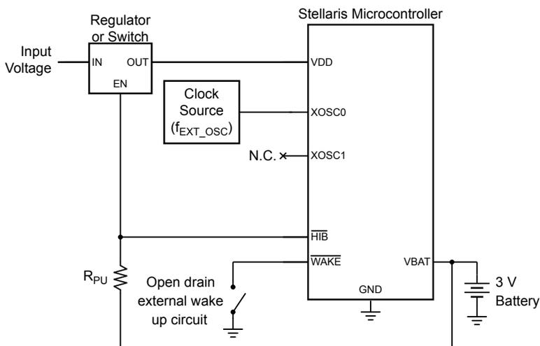
**Note:**  $R_{PU}$  = Pull-up resistor (1 M $\Omega$ ).
