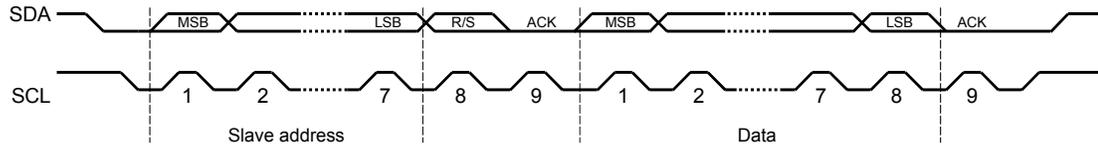
The first seven bits of the first byte make up the slave address (see Figure 13-5 on page 472). The eighth bit determines the direction of the message. A zero in the R/S position of the first byte means that the master will write (send) data to the selected slave, and a one in this position means that the master will receive data from the slave.
