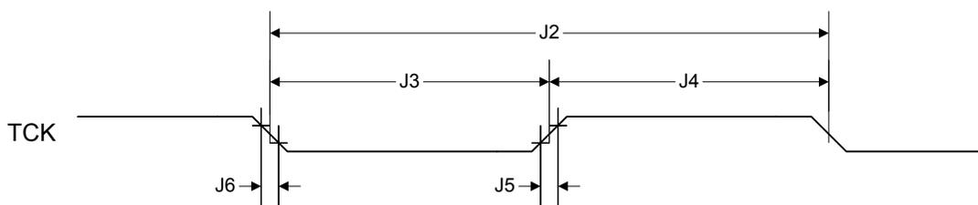
Figure 19-3. JTAG Test Access Port (TAP) Timing
