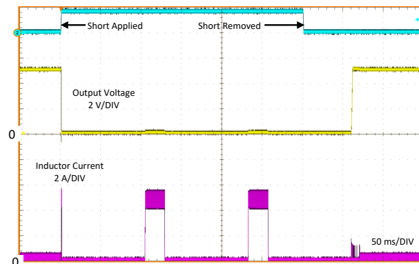
Figure 7-13. Short-Circuit Transient and Recovery
