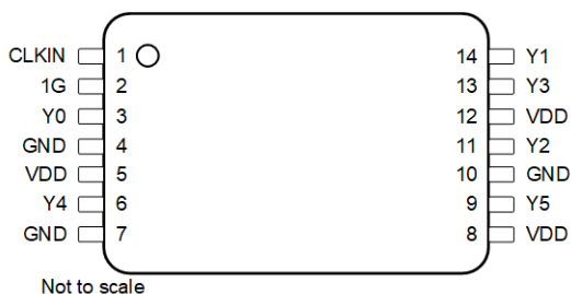
Figure 5-3. LMK1C1106-Q1, 14-Pin PW TSSOP Package (Top View)
