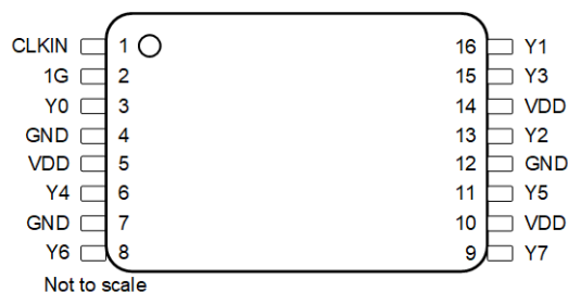
Figure 5-4. LMK1C1108-Q1, 16-Pin PW TSSOP Package (Top View)
