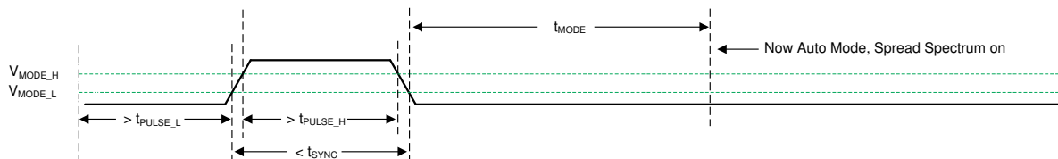
Figure 7-5. Transition from SYNC Mode to Auto Mode
