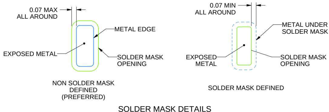
LAND PATTERN EXAMPLE EXPOSED METAL SHOWN SCALE: 20X
