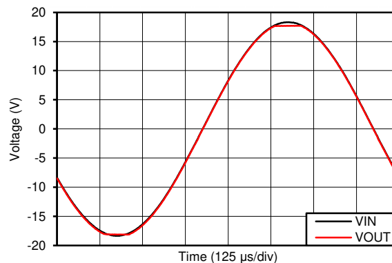
Figure 31. Output Waveform Devoid of Phase Reversal During an Input Overdrive Condition
