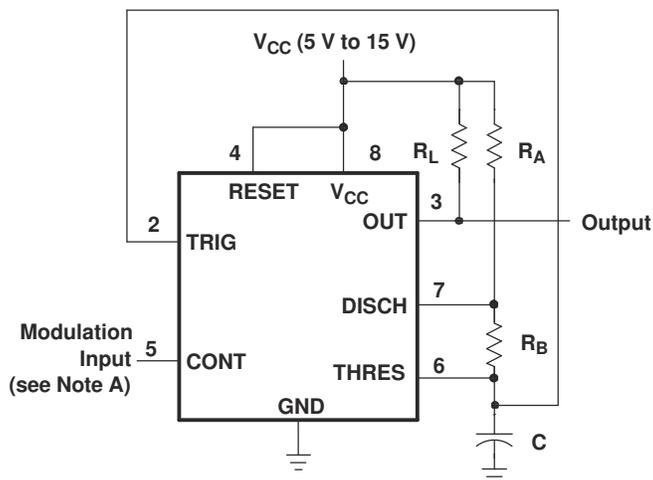
Pin numbers shown are for the D, JG, P, PS, and PW packages.
