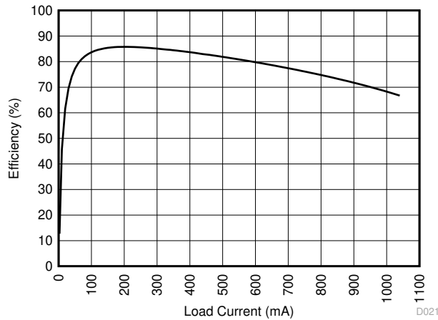
SN6505B + Würth 750316028 V_{CC} = 3.3\text{ V}
