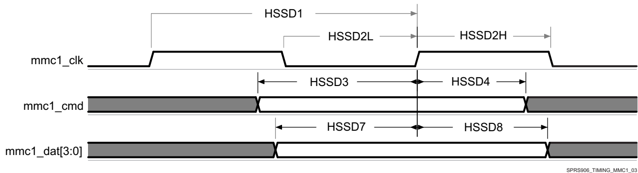
Figure 5-72. MMC/SD/SDIO in - High Speed - Receiver Mode
