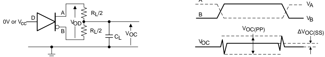
Figure 12. Measurement of Driver Differential and Common-Mode Output With RS-485 Load
