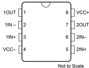
**Figure 3-2. TL052 D, P, or PS Package, 8-Pin SOIC, PDIP, or SOP (Top View)**
