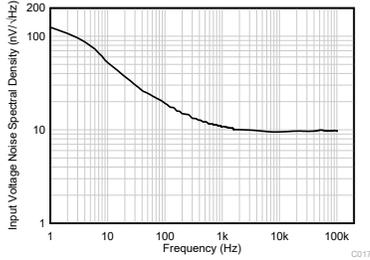
Figure 4-11. Equivalent Input Noise Voltage vs Frequency
