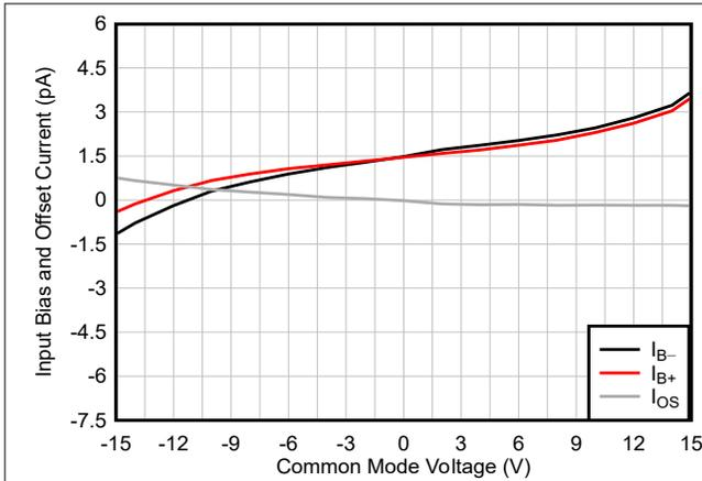
**Figure 4-1. Input Bias Current vs Common-Mode Input Voltage**
