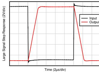
Figure 4-15. Voltage-Follower Large-Signal Pulse Response
