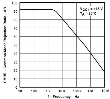
**Figure 4-4. Common-Mode Rejection Ratio vs Frequency**
