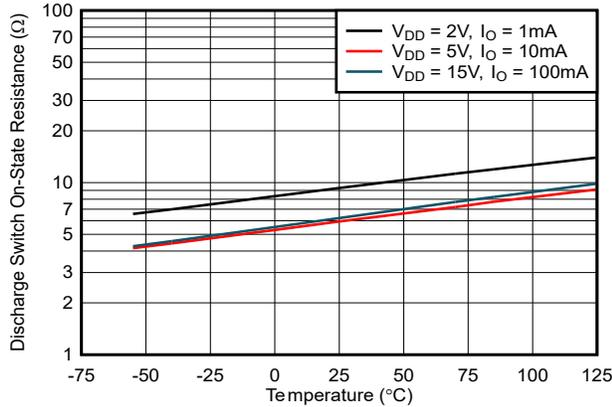
**Figure 5-1. Discharge Switch On-State Resistance vs Free-Air Temperature**
