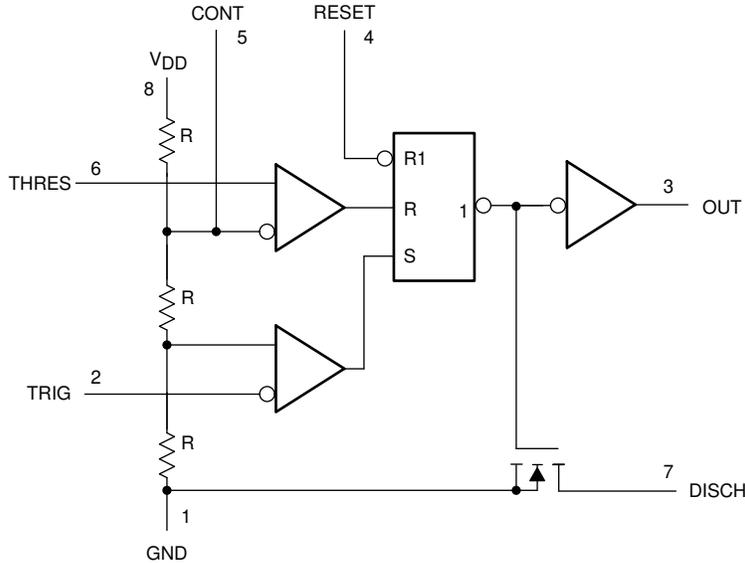
Pin numbers are for all packages except PW and FK. RESET overrides TRIG, which overrides THRES (when CONT pin is  $2/3 V_{DD}$ ). The resistance of R resistors vary with  $V_{DD}$  and temperature. The resistors match each other very well across  $V_{DD}$  and temperature for a temperature-stable control-voltage ratio.
