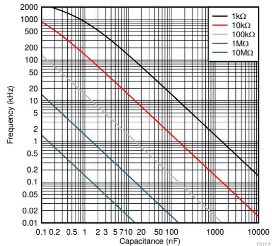
**Figure 6-8. Nominal Free-Running Frequency vs Timing Capacitance**
