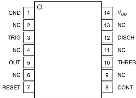
**Figure 4-2. PW Package, 14-Pin TSSOP (Top View)**
