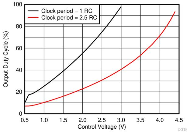
**Figure 7-4. Pulse-Width-Modulation vs Control Voltage**
