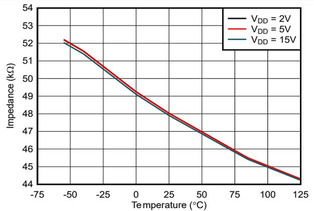
**Figure 5-4. Control Impedance vs Temperature**
