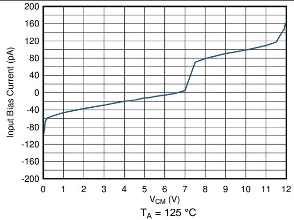
Figure 10. Input Bias Current vs. Common Mode, 125°C
