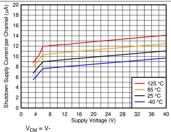
Figure 14. Shutdown Supply Current vs. Supply Voltage
