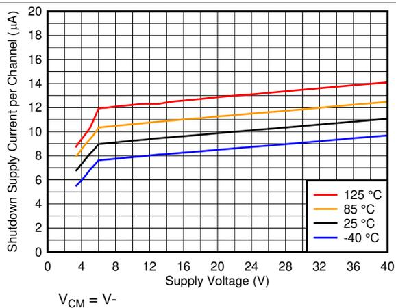
Figure 13. Shutdown Supply Current vs. Supply Voltage
