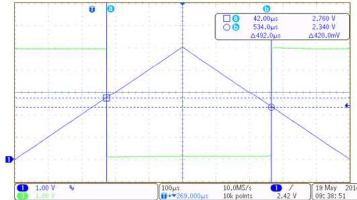
Figure 67. TLV1805 Upper and Lower Threshold with Hysteresis
