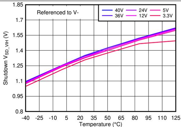
Figure 15. Shutdown Voltage High Threshold vs. Temperature
