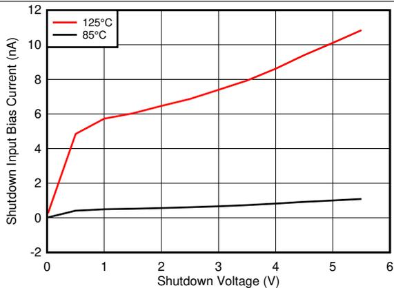
Figure 19. Shutdown Input Bias Current vs. Shutdown Input Voltage, High Temperatures
