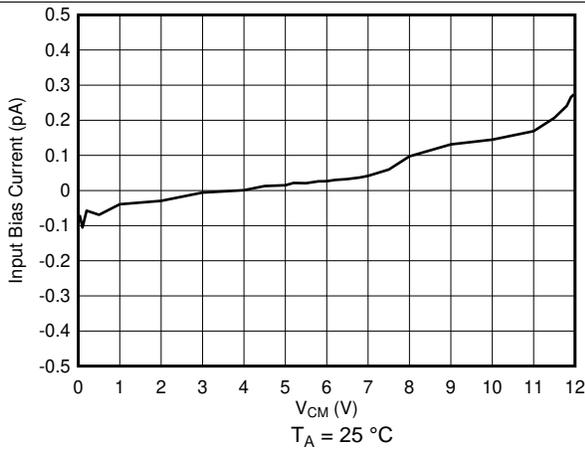
Figure 11. Input Bias Current vs. Common Mode, 25°C
