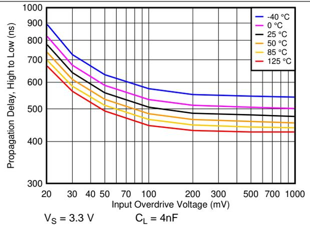
Figure 44.  $T_{PHL}$  Response Time vs. Overdrive at 3.3V
