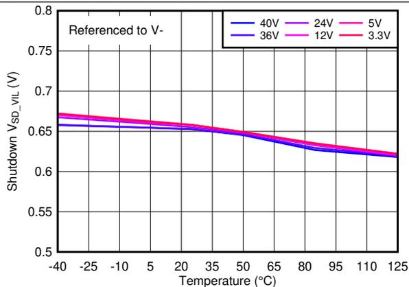
Figure 16. Shutdown Voltage Low Threshold vs. Temperature
