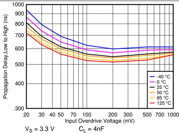
Figure 43.  $T_{PLH}$  Response Time vs. Overdrive at 3.3V
