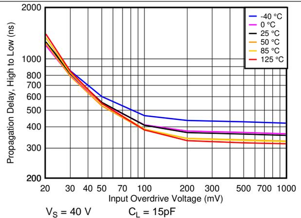
Figure 42.  $T_{PHL}$  Response Time vs. Overdrive at 40V
