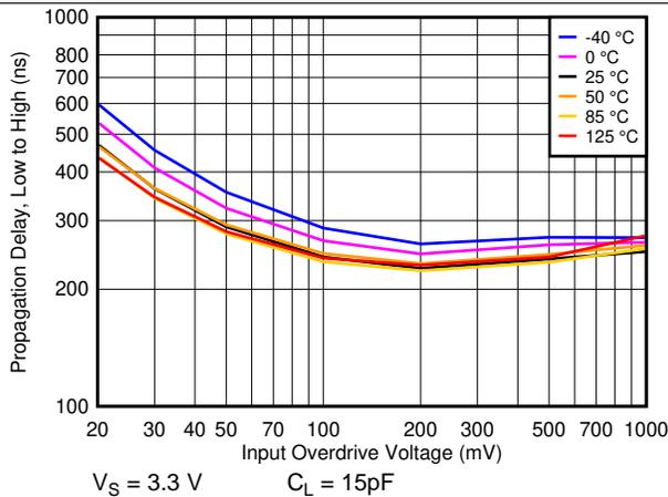
Figure 35.  $T_{PLH}$  Response Time vs. Overdrive at 3.3V
