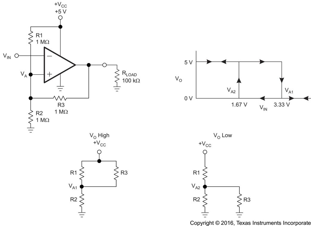
Figure 64. TLV1805 in an Inverting Configuration With Hysteresis
