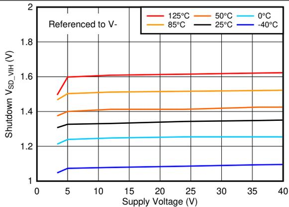
Figure 17. Shutdown Voltage High Threshold vs. Supply Voltage
