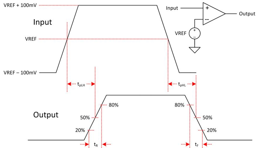
**Figure 1. Propagation Delay**
