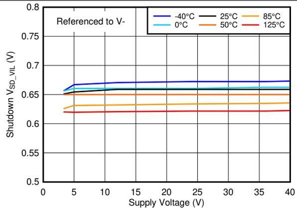
Figure 18. Shutdown Voltage Low Threshold vs. Supply Voltage
