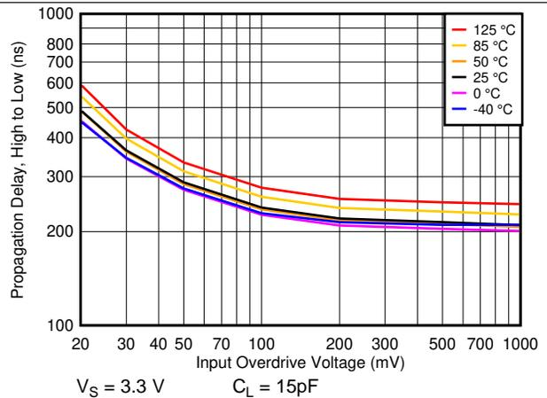
Figure 36.  $T_{PHL}$  Response Time vs. Overdrive at 3.3V
