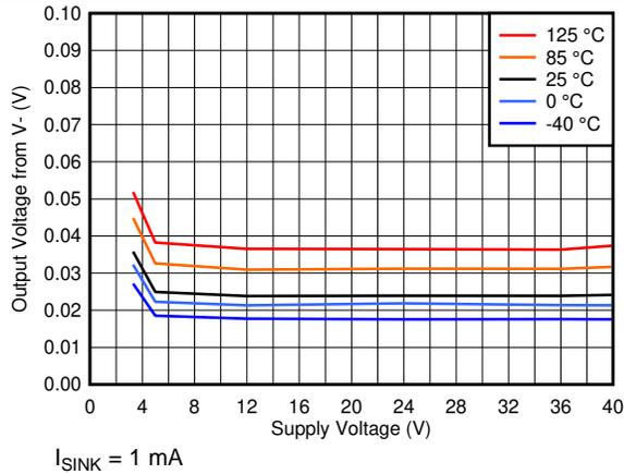
Figure 23. Output Low Voltage vs. Supply Voltage
