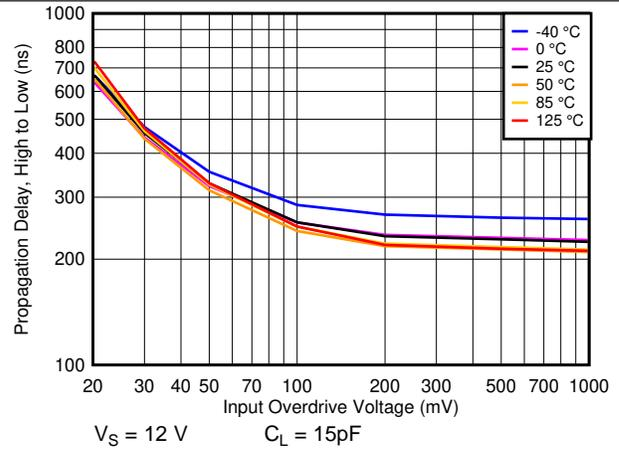
Figure 40.  $T_{PHL}$  Response Time vs. Overdrive at 12V
