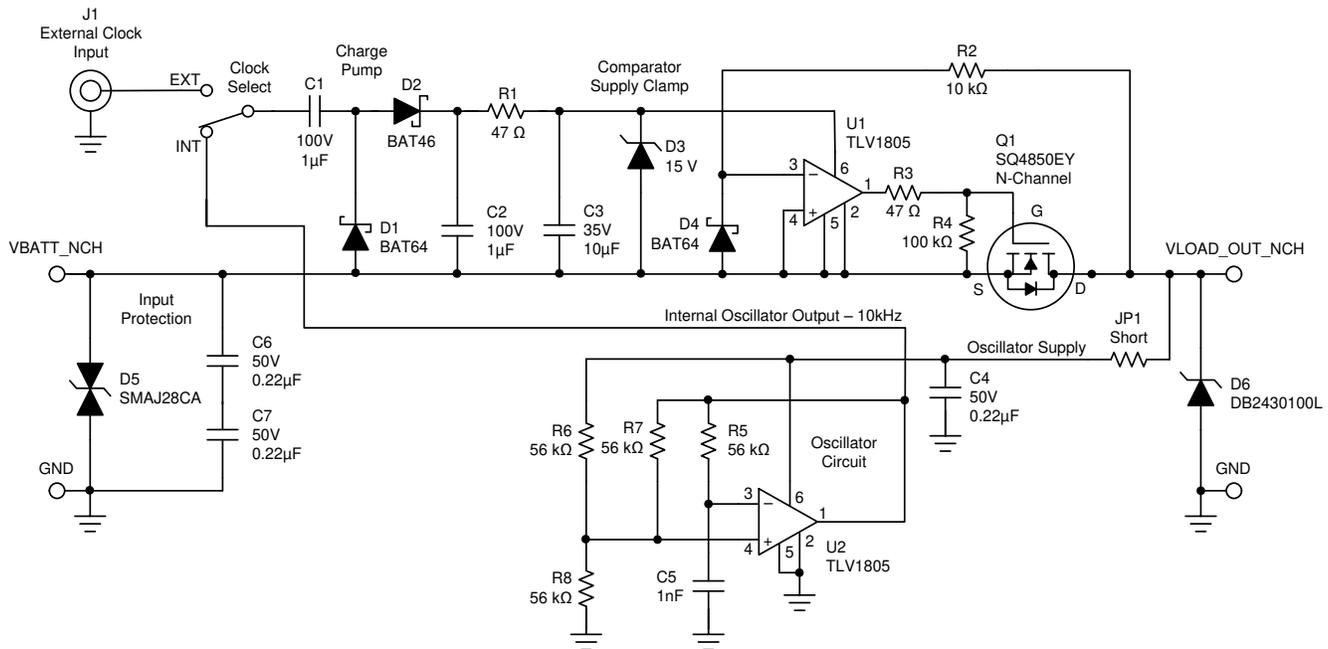
**Figure 69. N-Channel Reverse Current Schematic with Oscillator**
