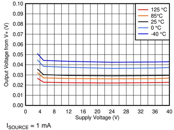
Figure 24. Output High Voltage vs. Supply Voltage
