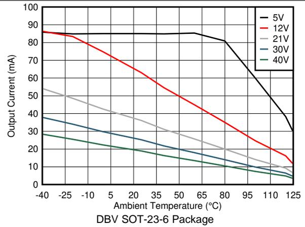
Figure 22. Maximum Continuous Output Current vs. Ambient Temperature
