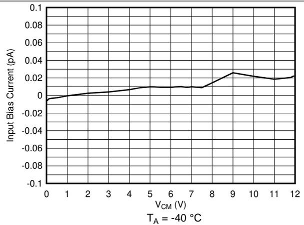
Figure 12. Input Bias Current vs. Common Mode, -40°C
