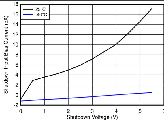
Figure 20. Shutdown Input Bias Current vs. Shutdown Input Voltage, Low Temperatures
