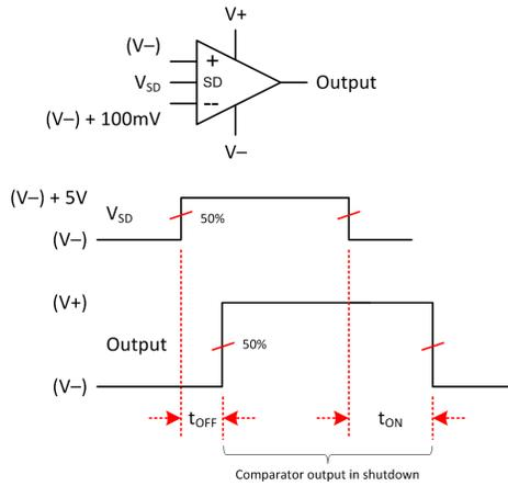
**Figure 2. Shutdown Timing**
