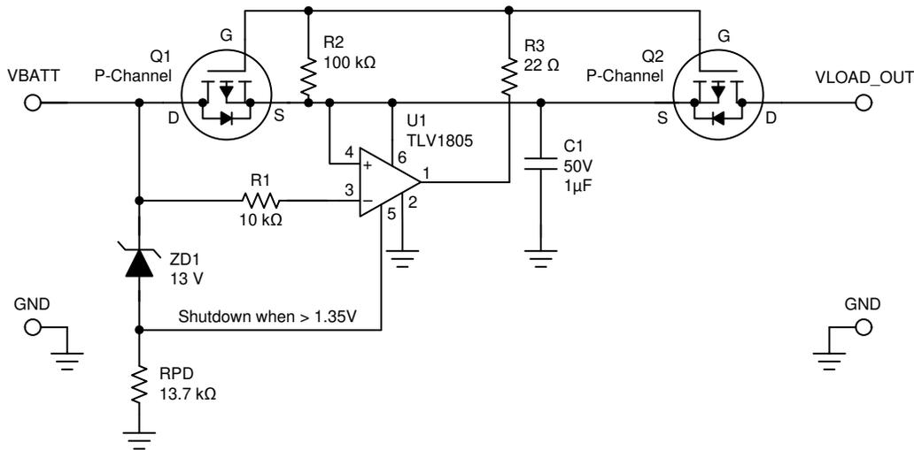
**Figure 71. Adding Overvoltage Protection Using SHDN Pin**
