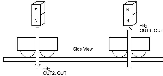
**Figure 7-2. Magnetic Flux Density Axis of Sensitivity**
