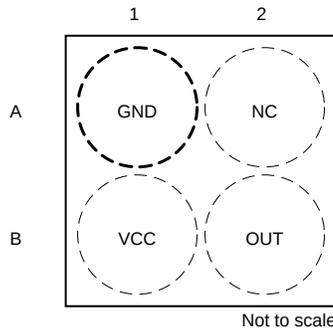
Figure 5-1. YBK Package 4-Pin DSBGA (Omnipolar) Top View
