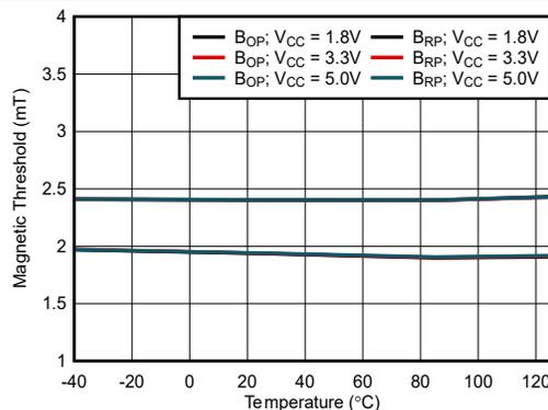
Figure 6-6. 15mT B<sub>OP</sub>, 13mT B<sub>RP</sub>: Thresholds vs Temperature
