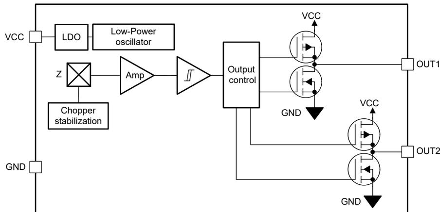
**Figure 7-1. Block Diagram**
