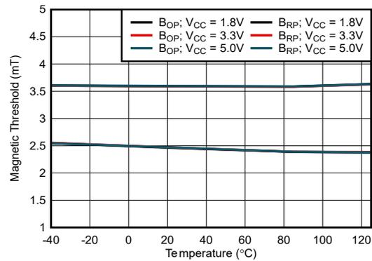
Figure 6-2. 3.5mT B<sub>OP</sub>: Thresholds vs Temperature
