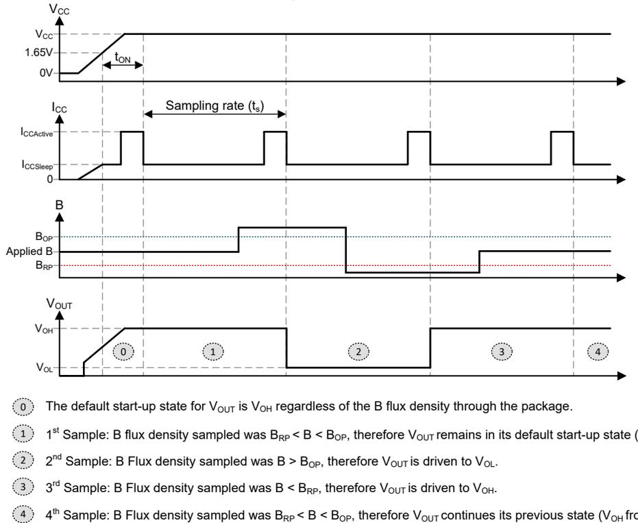
**Figure 7-7. Timing and Output Diagram**
