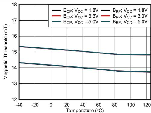
Figure 6-5. 15mT B<sub>OP</sub>, 14.1mT B<sub>RP</sub>: Thresholds vs Temperature
