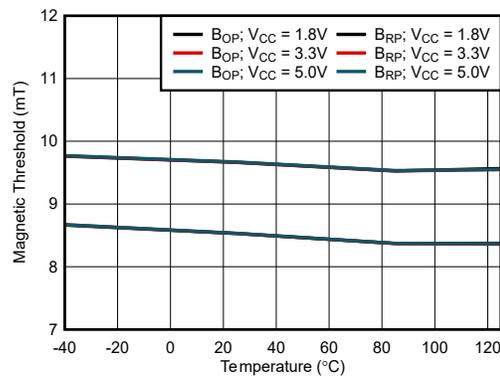
Figure 6-4. 9.5mT B<sub>OP</sub>: Thresholds vs Temperature
