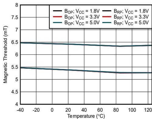
Figure 6-3. 6.3mT B<sub>OP</sub>: Thresholds vs Temperature
