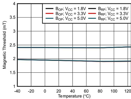
Figure 6-1. 2.4mT B<sub>OP</sub>: Thresholds vs Temperature
