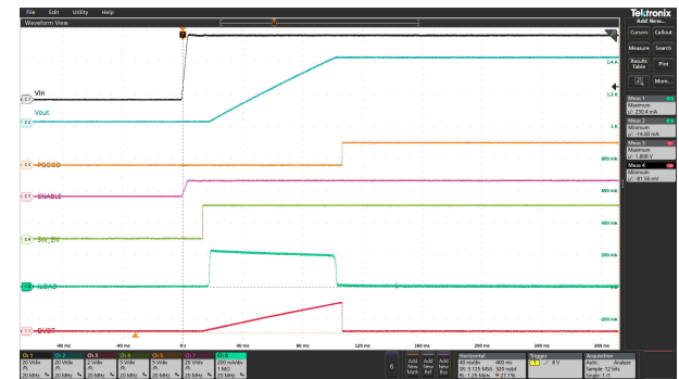
Input supply ramped up to 40V with appropriate resistor divider pulling EN high, C_{DVRT}=100\text{nF} , C_{OUT}=470\mu\text{F}
