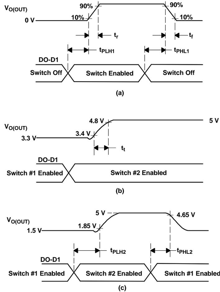
Figure 1. Propagation Delays and Transition Timing Waveforms
