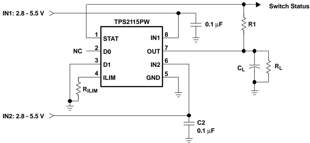
**Figure 13. Running a System From Two Battery Packs**
