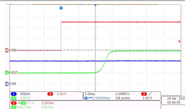
Figure 7-18. Turn-On at 1 V (CT = 1000 pF)
