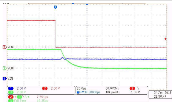
Figure 7-25. Turn-Off at 3.6 V
