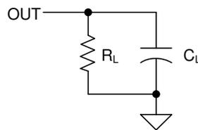
Figure 22. Output Rise / Fall Test Load
