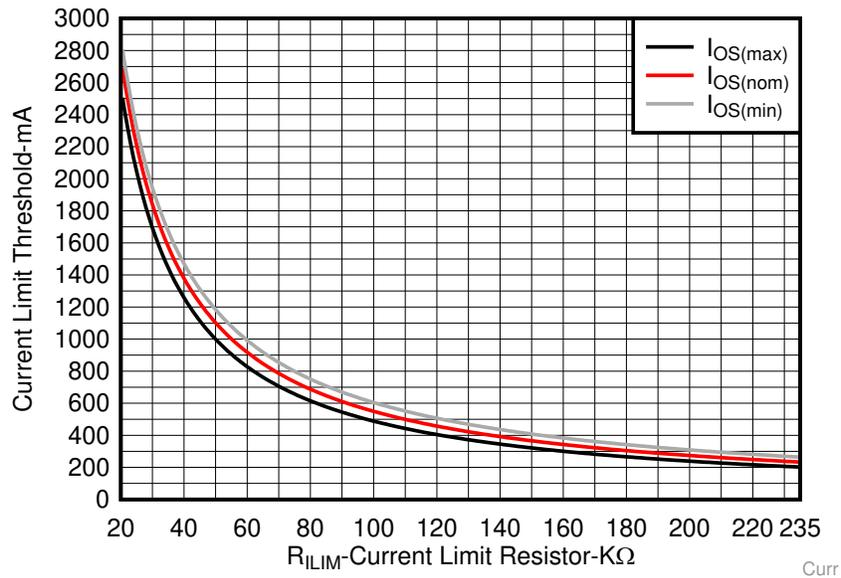
Figure 24. Current-Limit Threshold vs Current-Limit Resistor ( $R_{ILIM}$ )
