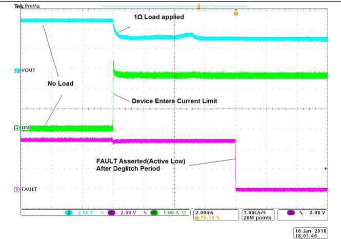
$V_{IN} = 5\text{ V}$ ,  $R_{ILIM} = 20\text{ k}\Omega$
