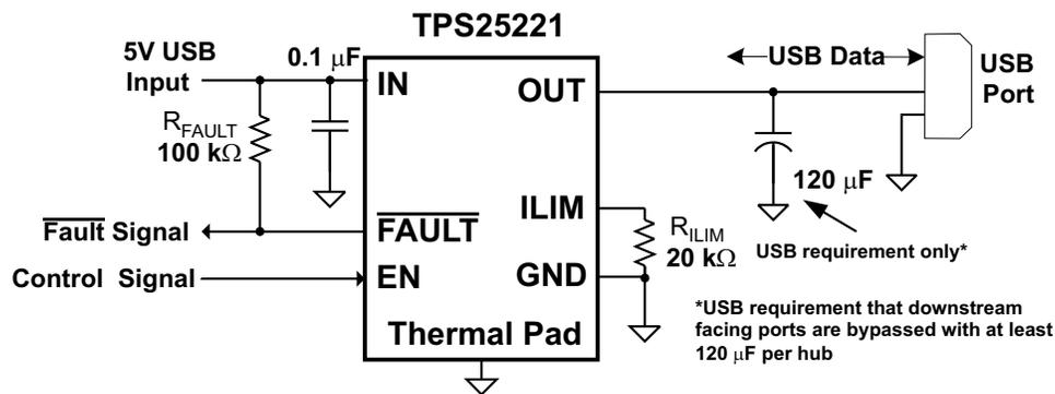
**Figure 29. Typical Application as USB Power Switch**
