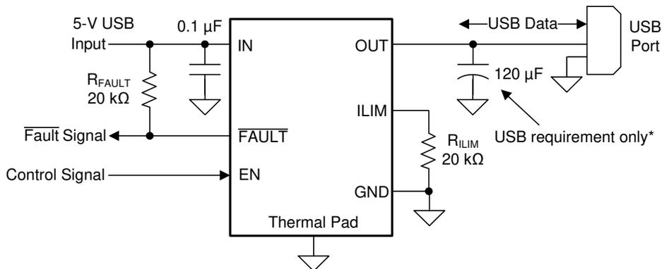
\*USB requirement that downstream facing ports are bypassed with at least 120  $\mu\text{F}$  per hub.
