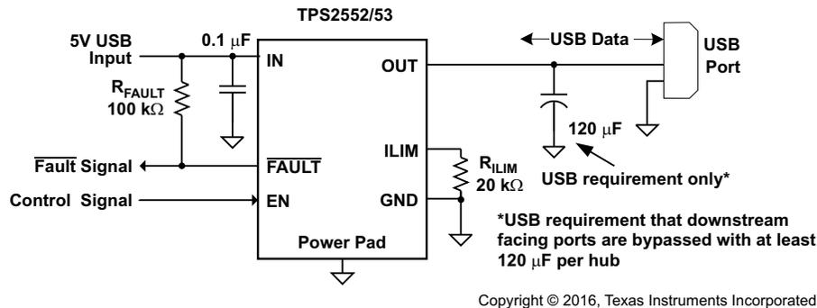
**Figure 29. Typical Application as USB Power Switch**
