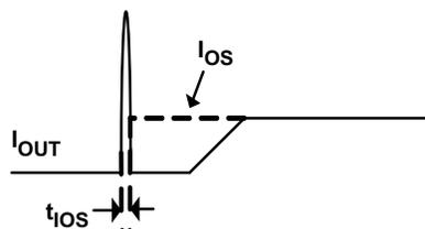
Figure 21. Response Time to Short-Circuit Waveform
