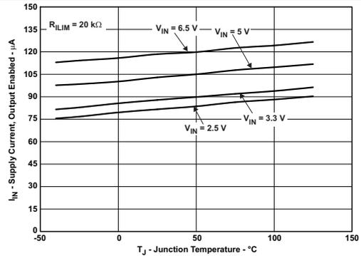
Figure 14.  $I_{IN}$  – Supply Current, Output Enabled –  $\mu A$
