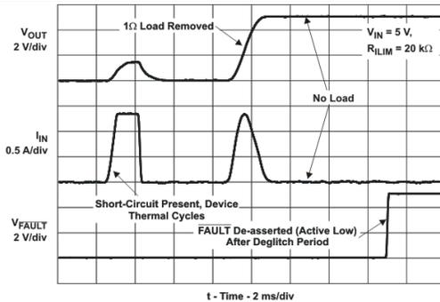
Figure 9. 1-Ω to No Load Transient Response
