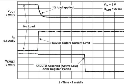
Figure 8. No Load to 1-Ω Transient Response
