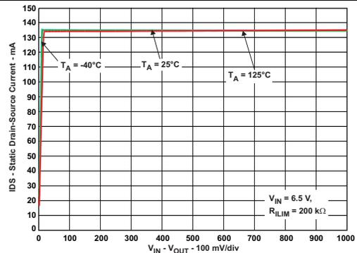
Figure 18. Switch Current Vs. Drain-Source Voltage Across Switch
