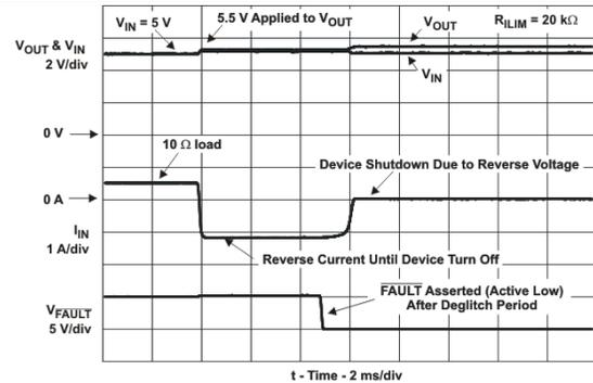
Figure 10. Reverse-Voltage Protection Response
