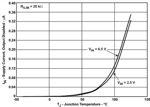
Figure 13.  $I_{IN}$  – Supply Current, Output Disabled –  $\mu A$
