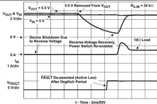
Figure 11. Reverse-Voltage Protection Recovery
