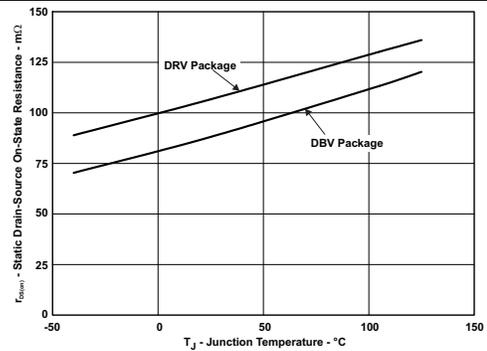
Figure 16. MOSFET  $r_{DS(on)}$  Vs. Junction Temperature
