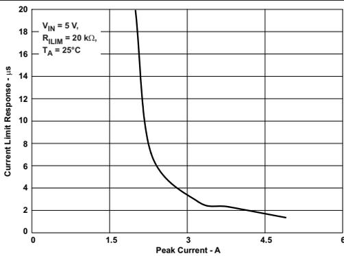
Figure 15. Current Limit Response –  $\mu s$
