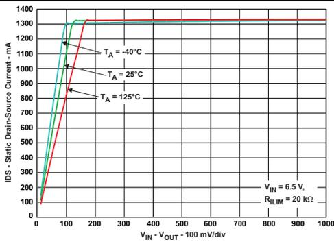
Figure 17. Switch Current Vs. Drain-Source Voltage Across Switch
