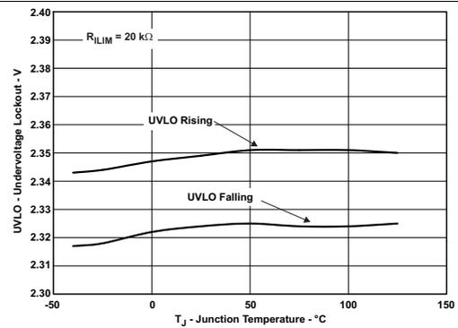
Figure 12. UVLO – Undervoltage Lockout – V
