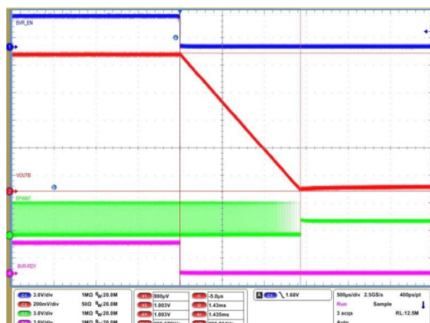
Figure 8-15. Soft-stop channel B (0 ms TOFF_DELAY)
