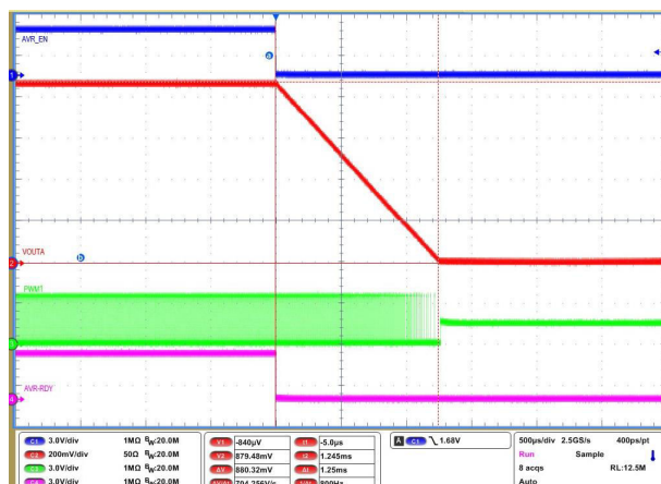
Figure 8-9. Soft-stop channel A (0 ms TOFF_DELAY)
