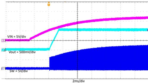
**Figure 7-16. TPS562203 Power On With 2A Loading**
