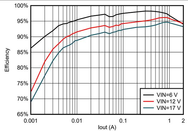
**Figure 5-16. TPS562203 Efficiency at 5 Vout With 4.7uH Inductor**
