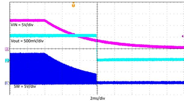
**Figure 7-17. TPS562203 Power Off With 2A Loading**
