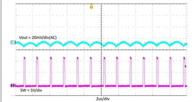
**Figure 7-10. TPS562203 Output Voltage Ripple With 2A Loading**
