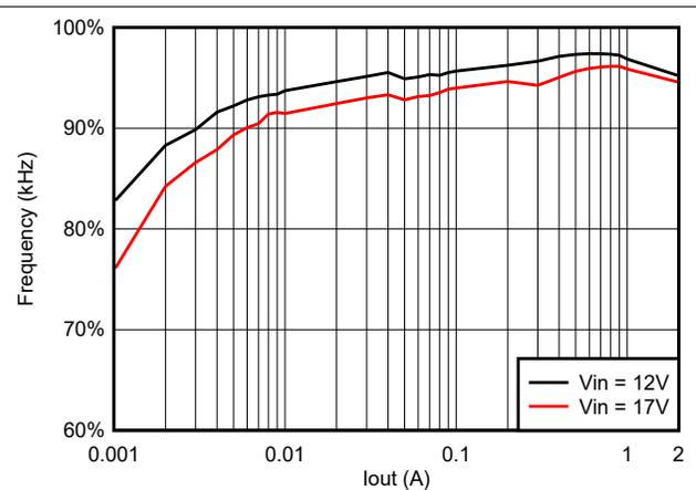
**Figure 5-18. TPS562203 Efficiency at 7 Vout With 6.8uH Inductor**
