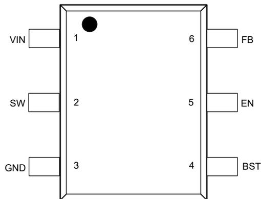
**Figure 4-1. 6-Pin SOT563 DRL Package (Top View)**
