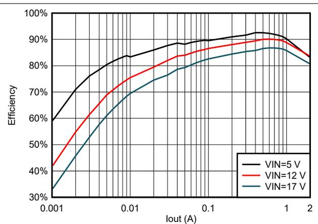
Figure 5-12. TPS562203 Efficiency at 1.05 Vout With 2.2uH Inductor
