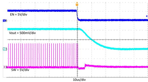
**Figure 7-15. TPS562206 Enable Off With 2A Loading**
