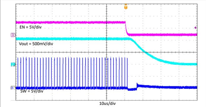
**Figure 7-13. TPS562203 Enable Off With 2A Loading**
