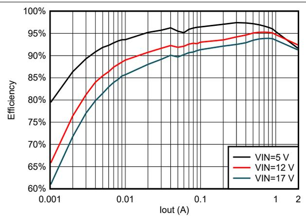
**Figure 5-14. TPS562203 Efficiency at 3.3 Vout With 4.7uH Inductor**
