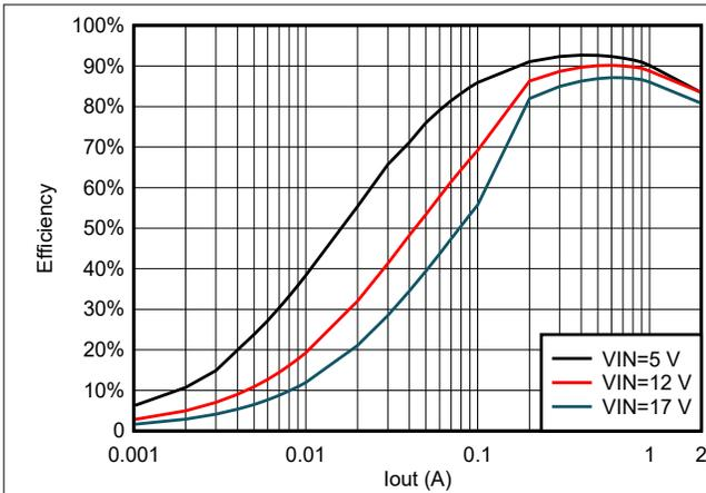
**Figure 5-13. TPS562206 Efficiency at 1.05 Vout With 2.2uH Inductor**
