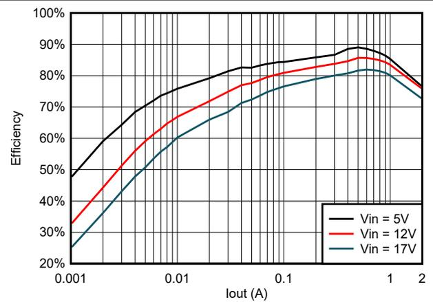
Figure 5-10. TPS562203 Efficiency at 0.6 Vout With 1.5uH Inductor
