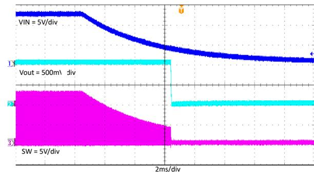
**Figure 7-19. TPS562206 Power Off With 2A Loading**
