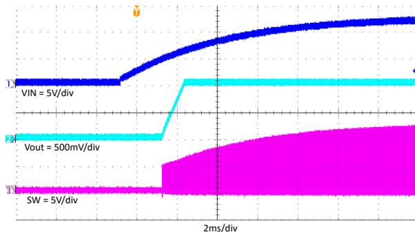
**Figure 7-18. TPS562206 Power On With 2A Loading**
