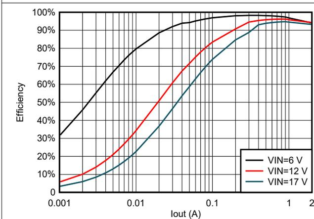
**Figure 5-17. TPS562206 Efficiency at 5 Vout With 4.7uH Inductor**
