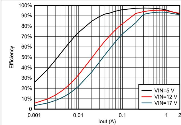
**Figure 5-15. TPS562206 Efficiency at 3.3 Vout With 4.7uH Inductor**
