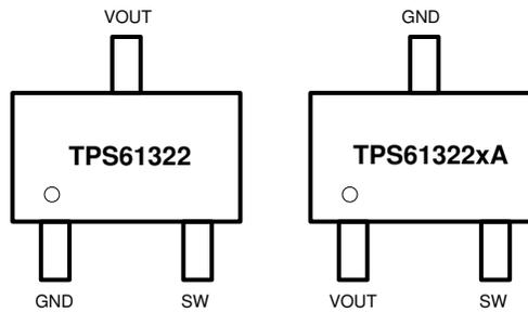
Figure 5-1. DBZ Package 3-Pin SOT Top View
