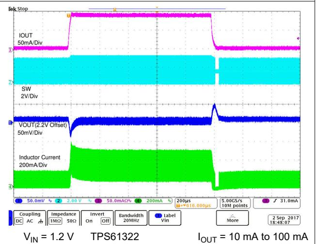
Figure 8-7. Load Transient
