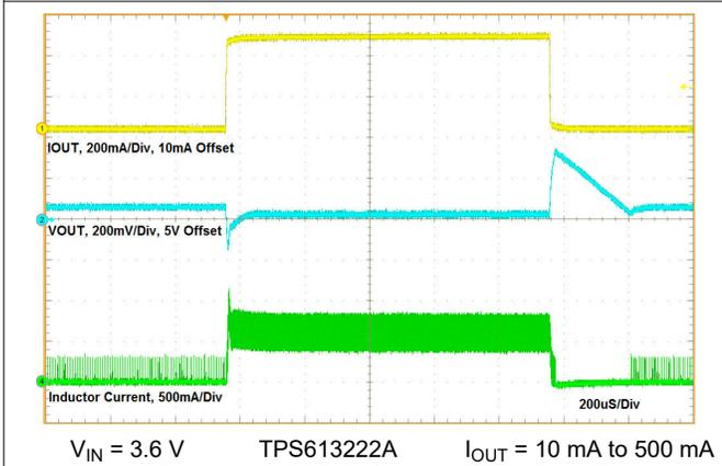
**Figure 8-16. Load Transient**
