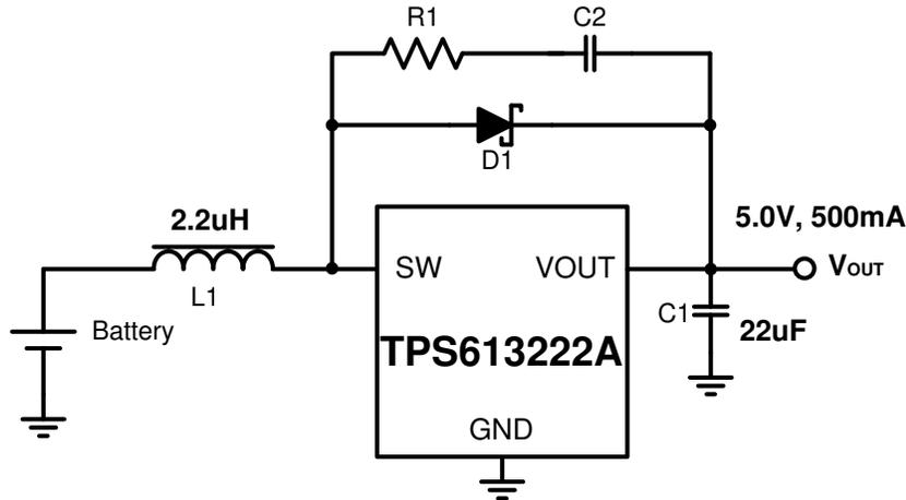
Figure 8-9. Typical Application Circuit with Schottky Diode
