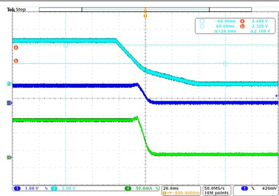
Channel 1 =  $V_{OUT}$ , channel 2 =  $V_{IN}$ , channel 4 =  $I_{OUT}$
