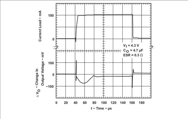
**Figure 7-13. TPS76933 Load Transient Response (Legacy Chip)**
