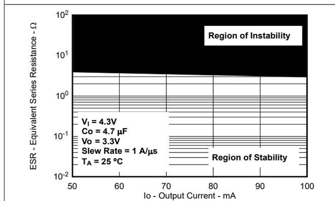
**Figure 5-50. Typical Region of Stability ESR vs Output Current (New Chip)**
