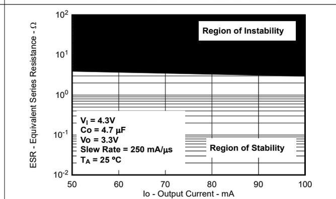
**Figure 5-51. Typical Region of Stability ESR vs Output Current (New Chip)**
