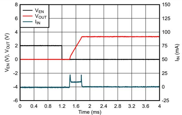
Figure 7-7. LDO Start-Up Time With EN (New Chip)
