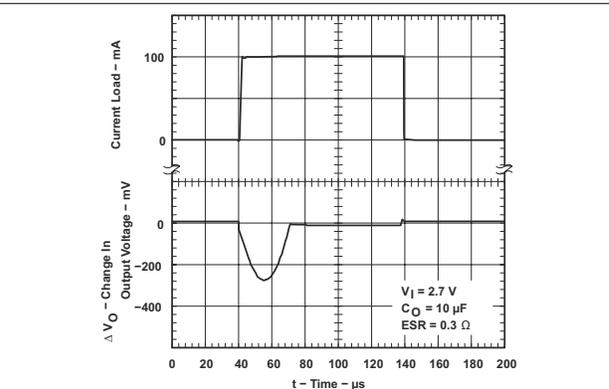
Figure 7-9. TPS76915 Load Transient Response (Legacy Chip)
