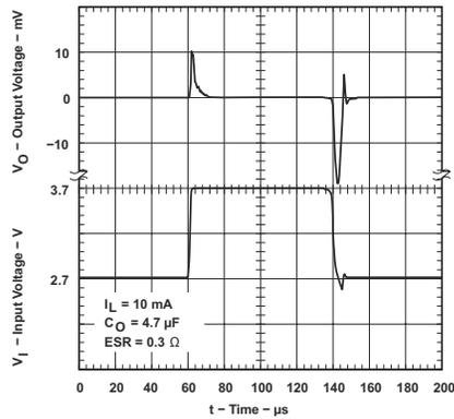
Figure 5-37. TPS76915 Line Transient Response (Legacy Chip)
