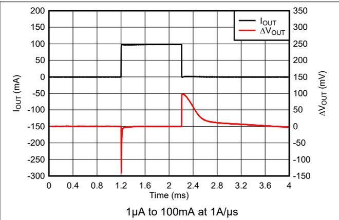
Figure 5-44. TPS76933 Load Transient Response (New Chip)
