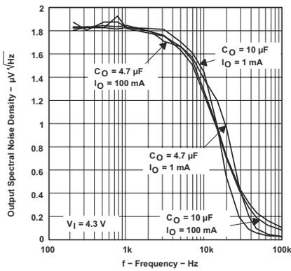
Figure 5-21. TPS76933 Output Spectral Noise Density vs Frequency (Legacy Chip)
