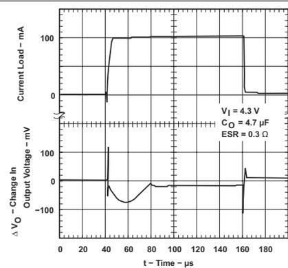
Figure 5-42. TPS76933 Load Transient Response (Legacy Chip)
