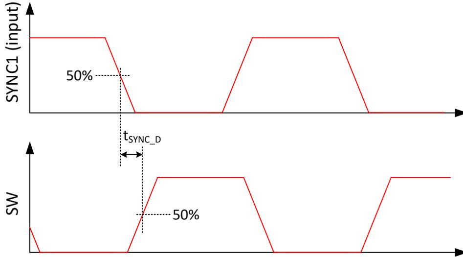
**Figure 8-6. SYNC1 to SW Delay: Inverted Sync**
