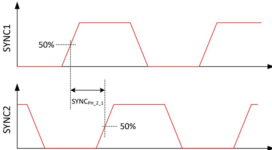
Figure 8-4. SYNC2 to SYNC1 Rising Edge Phase Shift
