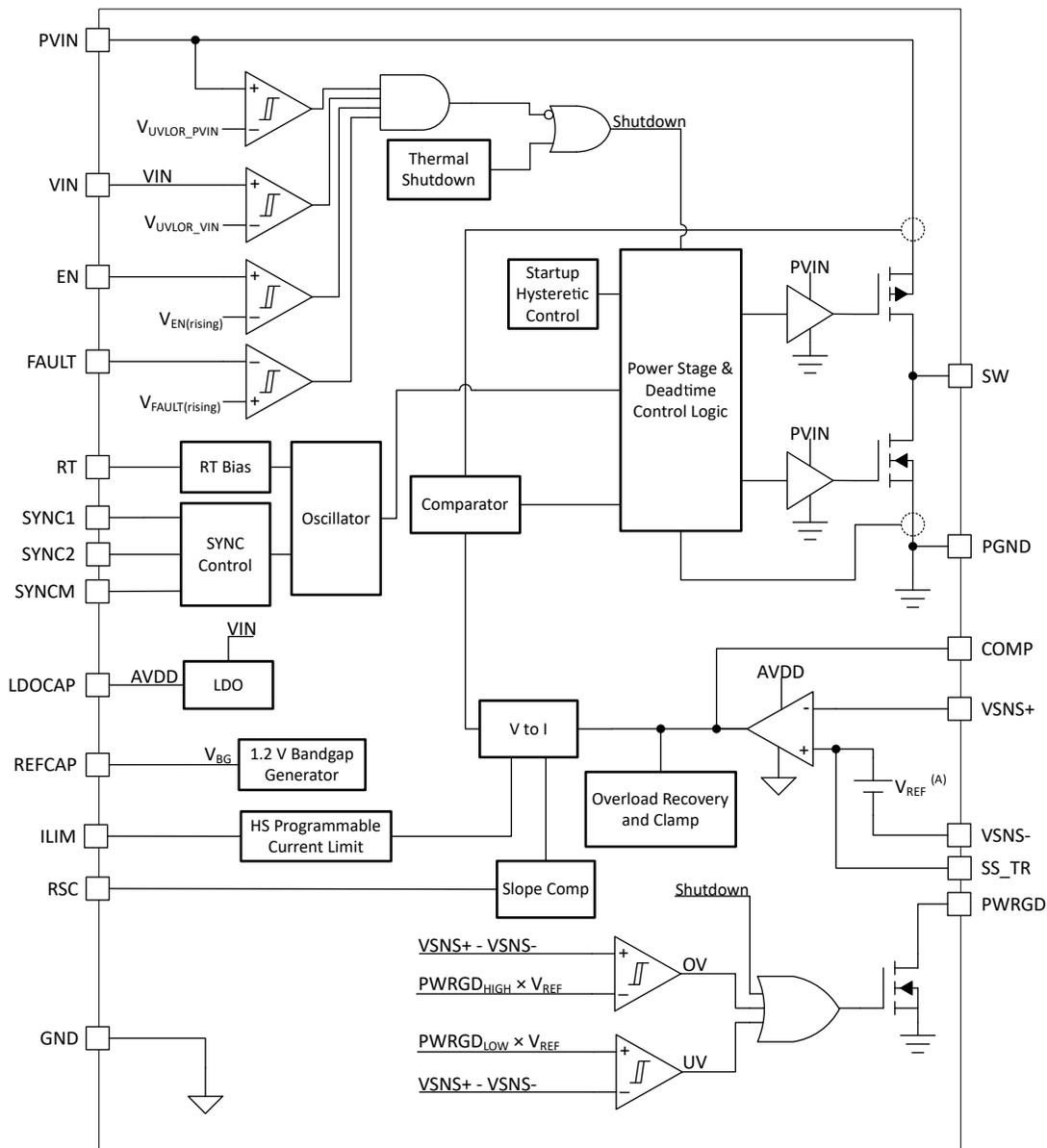
A.  $V_{REF}$  is a nominal 0.6V reference derived from the bandgap voltage; see [Section 9.3.2](#).
