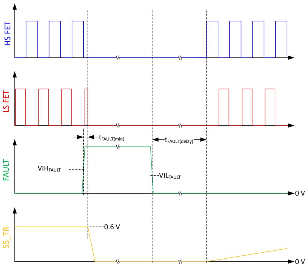
Figure 9-3. FAULT Pin Waveforms From External Signal
