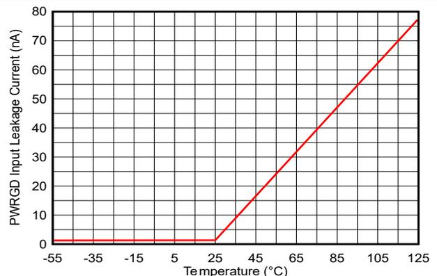
V<sub>SENSE</sub> = V<sub>REF</sub>, V<sub>PWRGD</sub> = 7V
