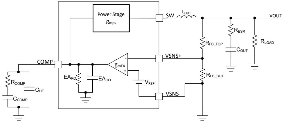
Figure 9-20. Simplified Small Signal Model For Loop Response
