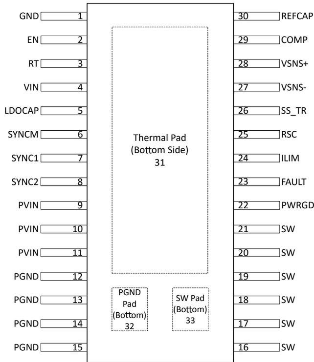
**Figure 6-1. HLB Package, 30-Pin CFP (Top View)**
