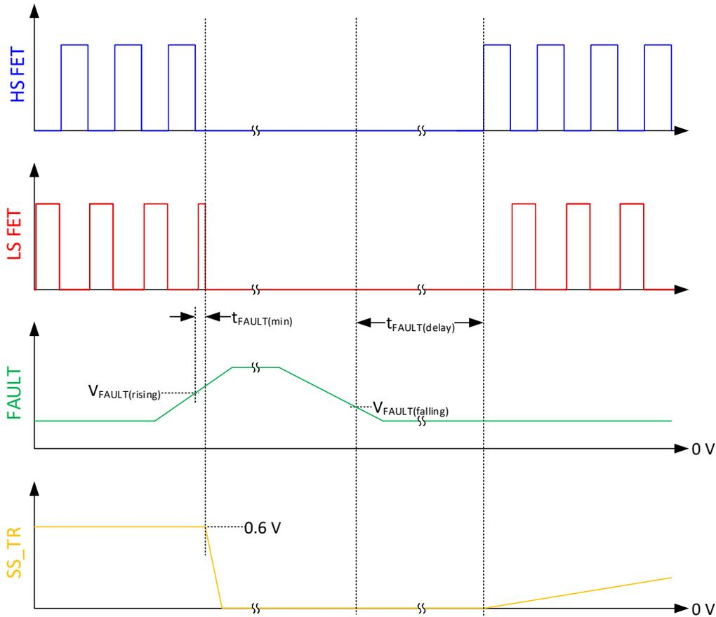
**Figure 9-4. FAULT Pin Waveforms From External Resistor Divider**
