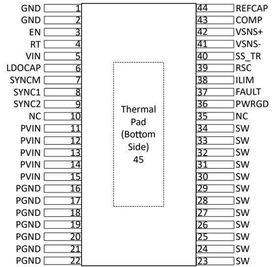
**Figure 6-2. DDW Package, 44-Pin HTSSOP (Top View)**
