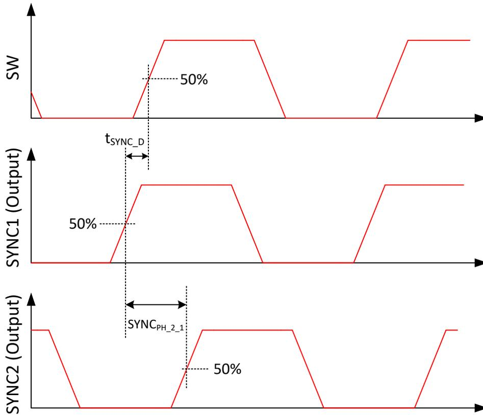
**Figure 8-7. SYNC1 to SW Delay: SYNC1 Output**
