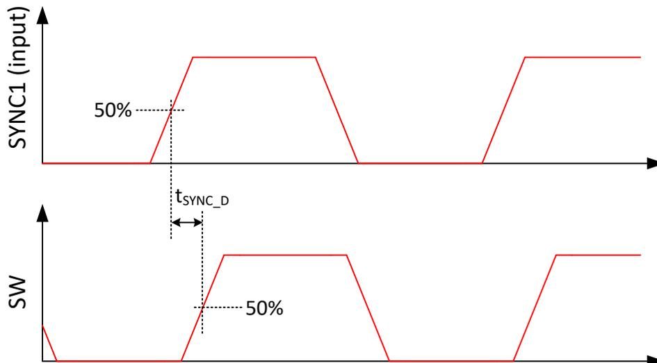
Figure 8-5. SYNC1 to SW Delay: Non-inverted Sync
