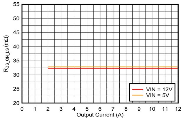
**Figure 7-61. Low Side FET Resistance vs Current**
