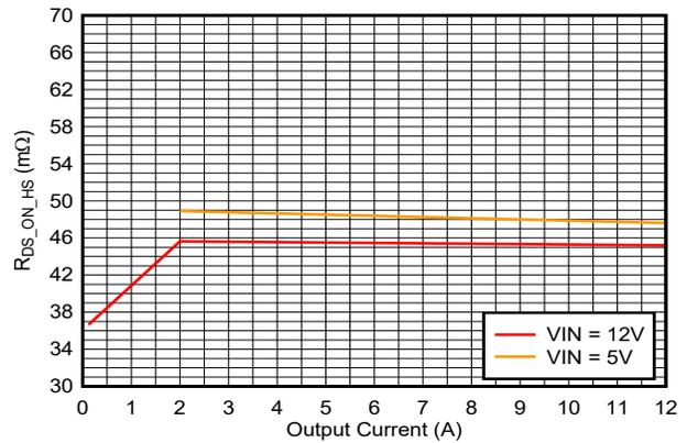
**Figure 7-60. High Side FET Resistance vs Current**
