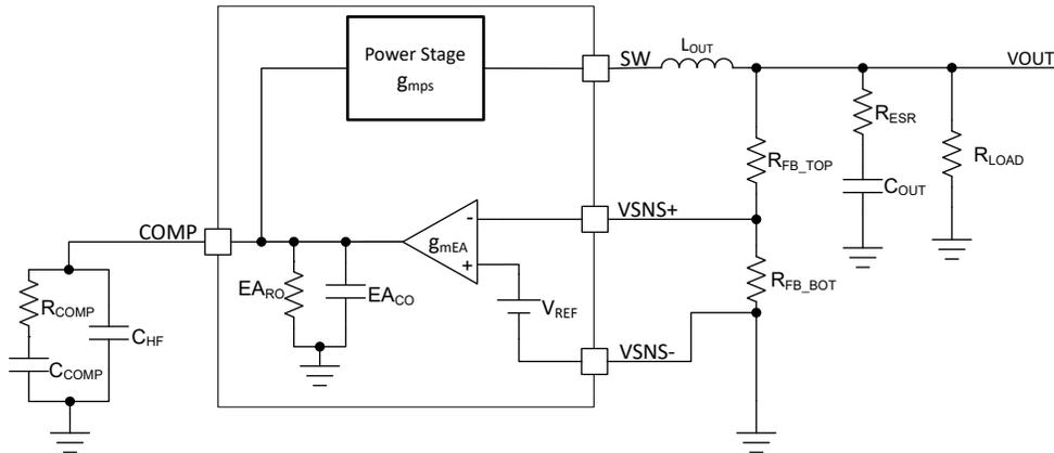
**Figure 10-2. Type II Compensation With Simplified Loop**
