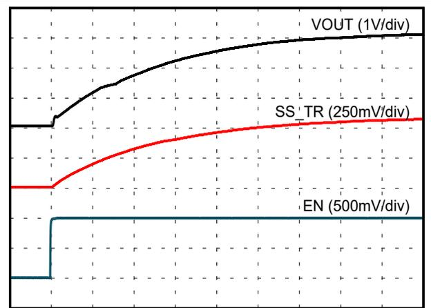
$I_{OUT} = 0A$ ,  $V_{OUT(set)} = 3.3V$ ,  $f_{SW} = 500kHz$ ,  $C_{OUT} = 1013\mu F$
