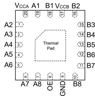
Figure 4-4. RUK Package (Top View)
