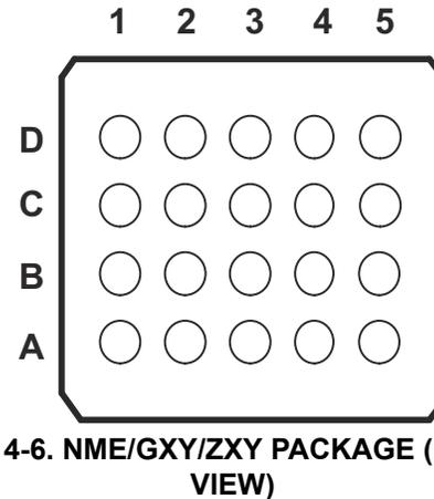
Figure 4-6. NME/GXY/ZXY PACKAGE (BOTTOM VIEW)
