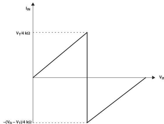
A.  $V_T$  is the input threshold voltage of the TXB0108 (typically  $V_{CC}/2$ ).
