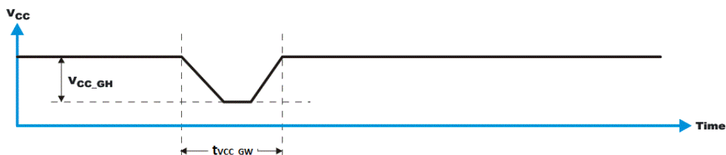
Figure 8-4. Glitch Width and Glitch Height
