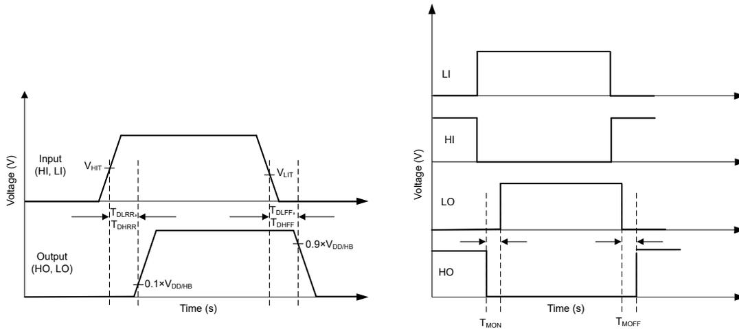
Figure 5-1. Timing Diagrams
