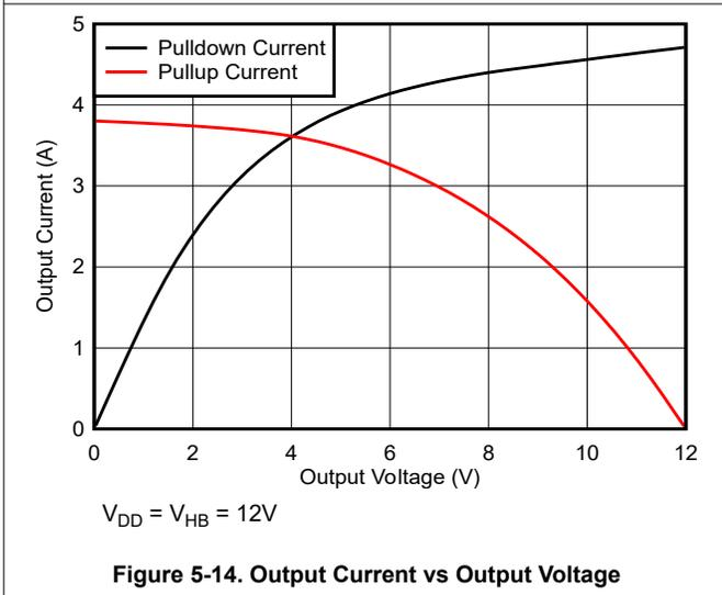
Figure 5-14. Output Current vs Output Voltage
