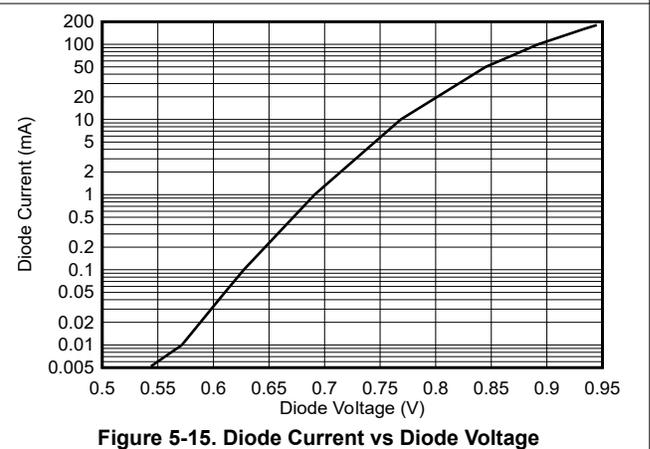
Figure 5-15. Diode Current vs Diode Voltage
