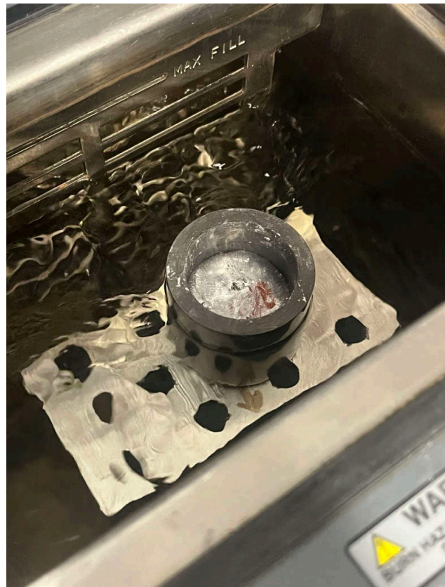
Figure 2-3. Crucible Filled with Liquid Gallium Placed in Oil Bath
