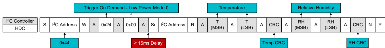
Figure 2-7. HDC302x Trigger-On Demand Communication Structure
