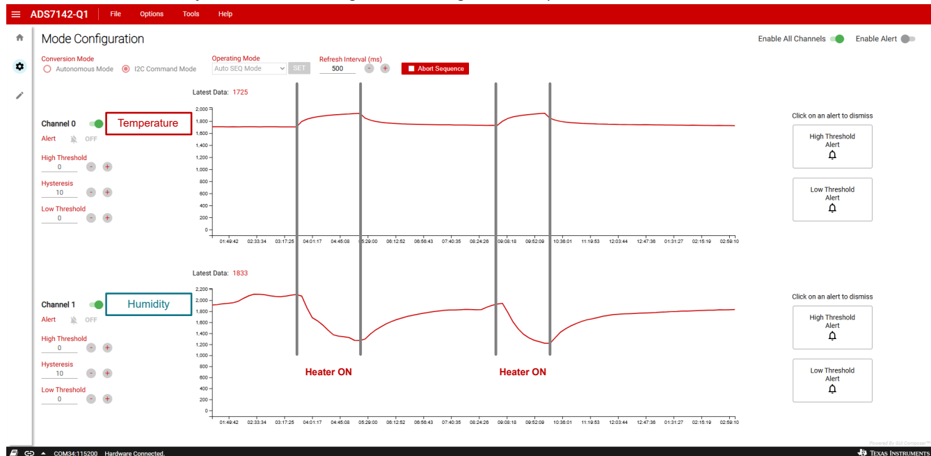
Figure 3-6. HDC3120 Output Interpretation With the BOOSTXL-ADS7142-Q1 EVM
