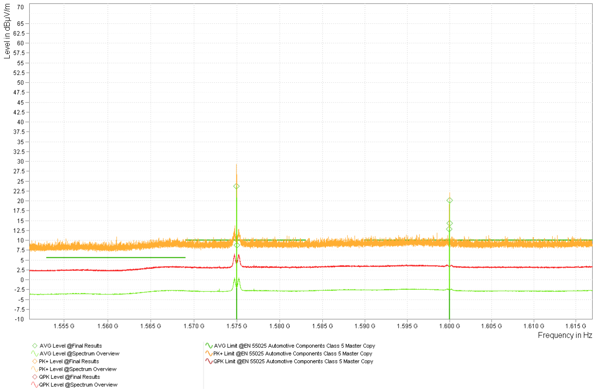
Figure 3-25. Variant 4 Competitor Oscillator 3.3V 1.5GHz to 1.6GHz Band Spectrum Overview - Horn
