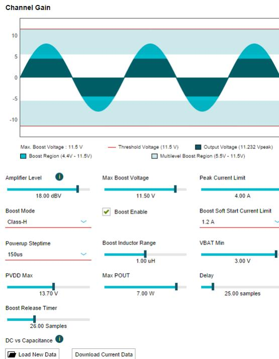
Figure 3-13. Playback and PCM PPC3 Configuration
