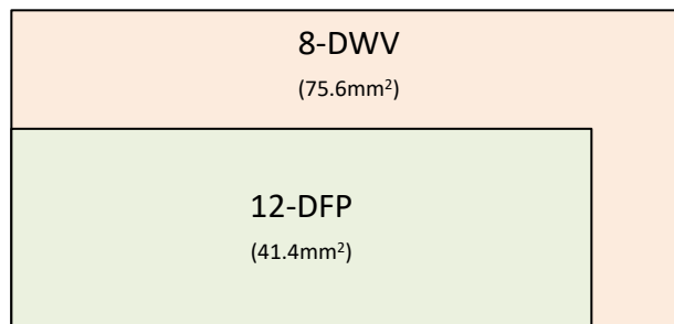
Figure 3-1. 2 Channel Digital ISO Area Comparison (mm 2 ): Traditional 8-DWV (Wide-SOIC) vs Small Form Factor 12-DFP (Wide-SSOP)
