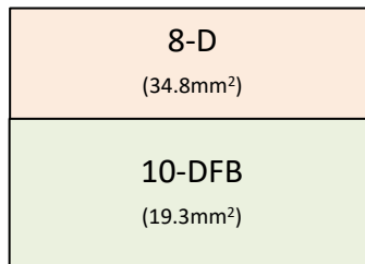
Figure 2-1. 2 Channel Digital ISO Area Comparison (mm 2 ): Traditional 8-D (SOIC) vs Small Form Factor 10-DFB (SSOP)
