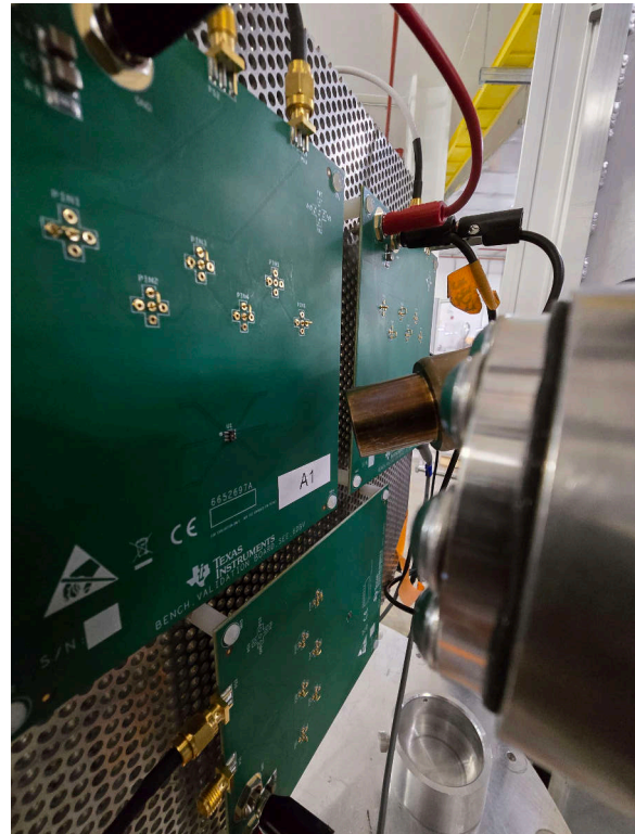
Figure 4-2. SN54SC1G08-SEP Evaluation Board at the MSU Facility (SET)
