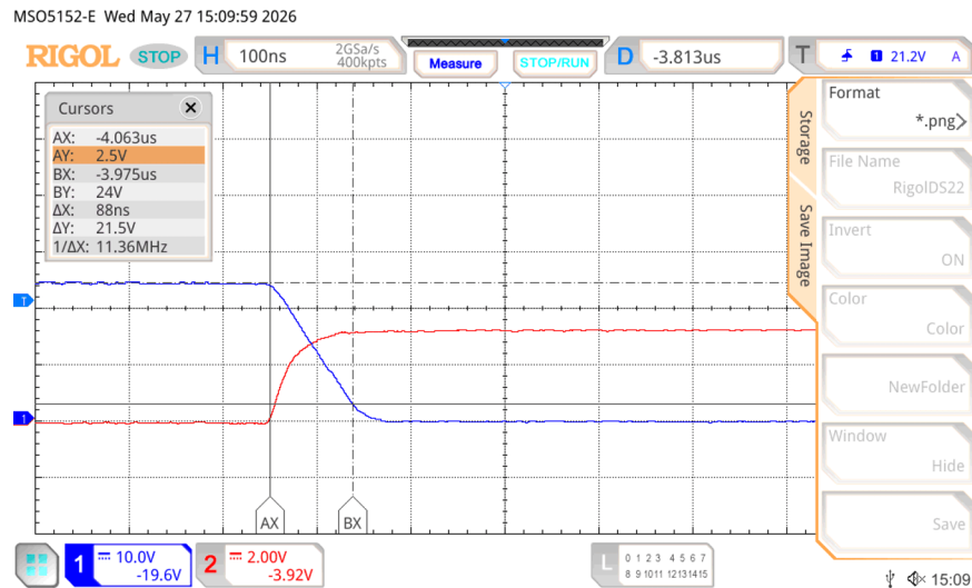
Figure 4-10. Turn-on Propagation Delay
