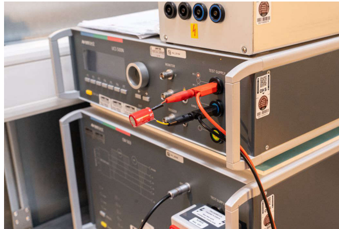
Figure 4-52. Additional Capacitance on Coupling Network
