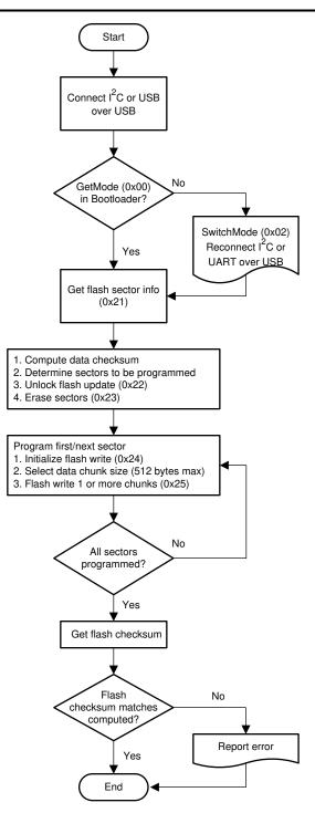
Figure 4-1. Flash Update Flow Diagram
