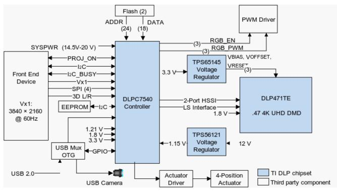
Figure 1-1. Typical Projector System Block Diagram
