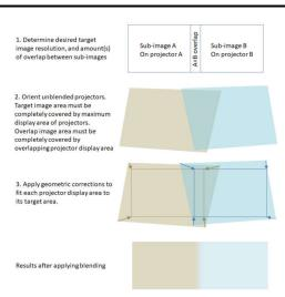
For Simple 1D RGB mode, warping is not allowed. Therefore, the projectors must be overlapped and orthogonally aligned. The overlaps between all projectors in the horizontal (X) direction and vertical direction (Y) are configurable. The gain and offset values for the blending map for any given projector within the blending system is directly determined by the user for Simple 1D RGB mode. For 2D Luminance mode, gain and offset are calculated from:
