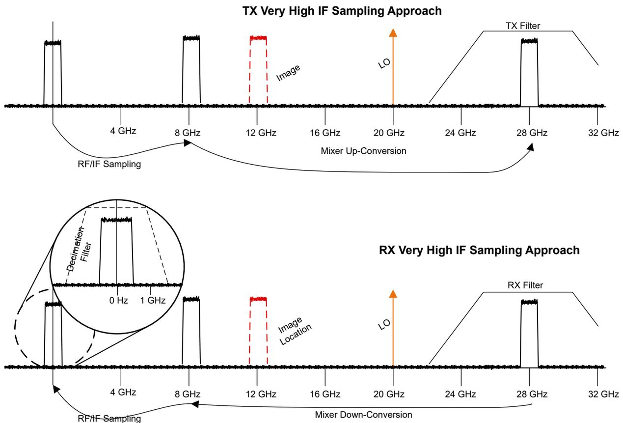
**Figure 3-1. AFE7950 in Super-het Architecture**
