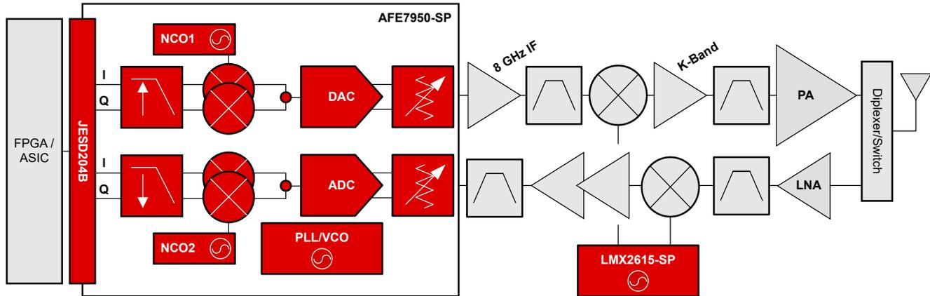
Figure 4-1. K-Band Super-het Block Diagram
