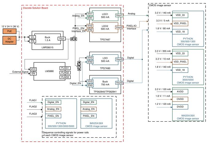
Figure 2-1. Block Diagram of Discrete Solution Board
