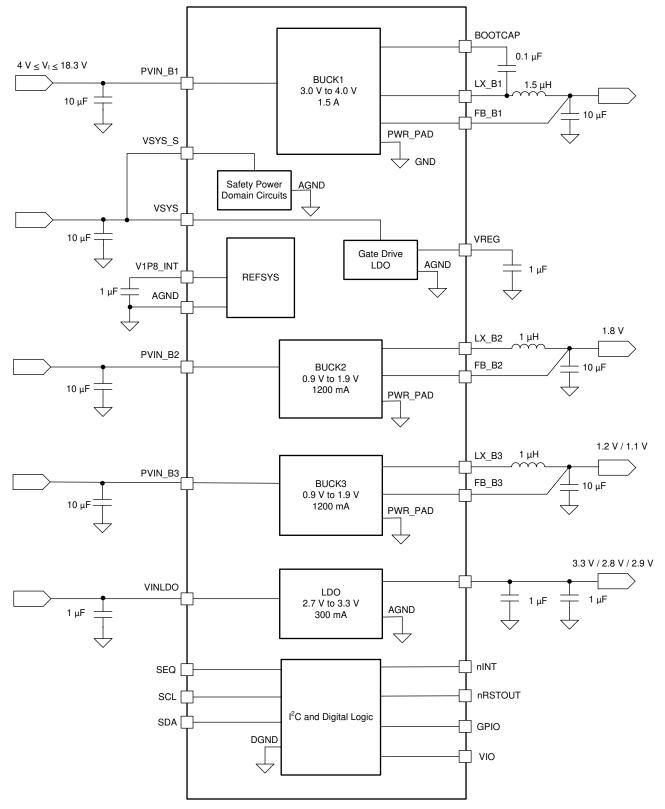
Figure 2-14. Block Diagram of the TPS650330-Q1
