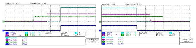
(b) Power Sequences of IMX25X/26X CMOS image sensors' power rails
