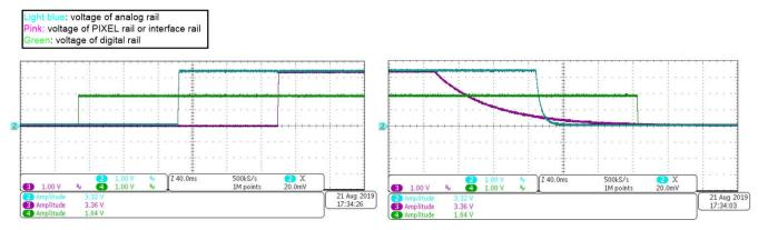
Figure 4-1. Power Sequence of the Power Rails of PYTHON 300/500/1300 CMOS Image Sensors Using the 120-ms Delay Time LM3880
