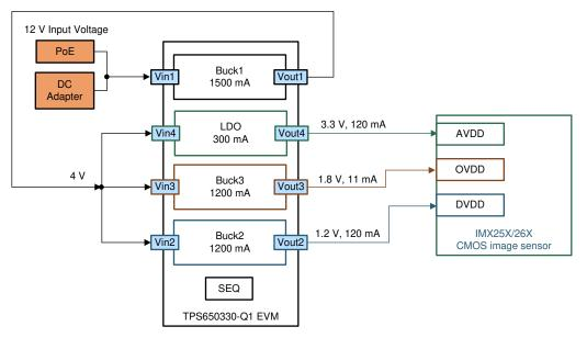
Figure 2-3. Block Diagram of PMIC TPS650330-Q1 Solution
