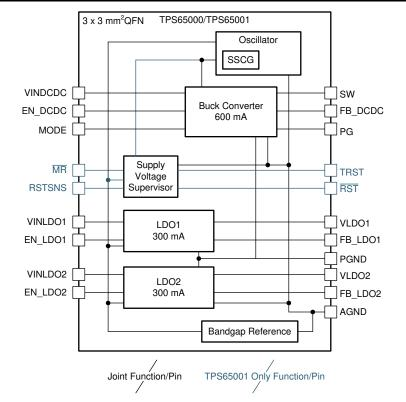
Figure 2-13. Block Diagram of the TPS65000
