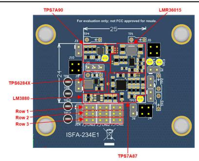
Figure 2-12. PCB Board of Discrete Solution
