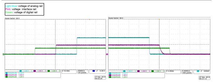
Figure 3-5. Power Sequences of the Power Rails of IMX25X/26X CMOS Image Sensors
