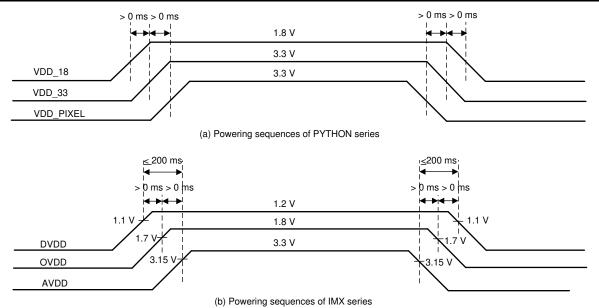
Figure 1-1. Specific Power Sequencing Needs
