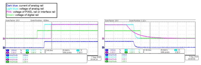
(a) Power Sequences of PYTHON 300/500/1300 CMOS image sensors' power rails
