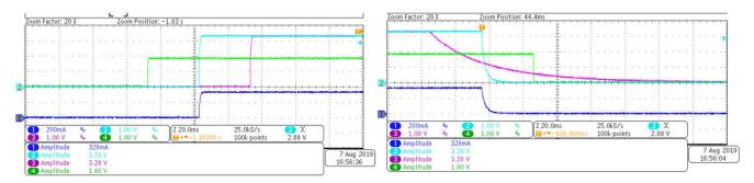
(b) Power Sequences of PYTHON 3000/5000 CMOS image sensors' power rails
