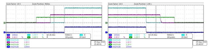
(c) Power Sequences of IMX25X/26X CMOS image sensors' power rails
