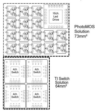
Figure 1-1. 16 Channel, 50V Solution Size Comparison (not drawn to scale)
