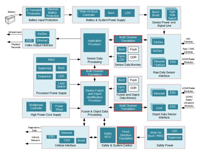
Figure 1. ADAS Domain Controller Reference Diagram and Common Level Translation Use Cases
