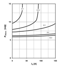
Figure 1. IPB072N15N3 Drain Source On-Resistance
