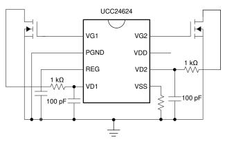
Figure 8. Adding RC Filter at VD Pins
