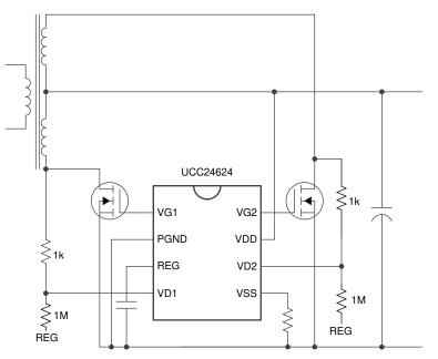
Figure 6. Decreasing Turn-off Threshold Circuit
