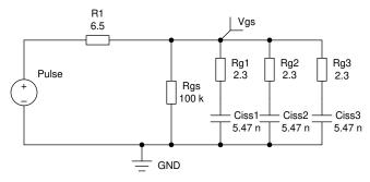
Figure 2. Driving Capability Simulation Circuit
