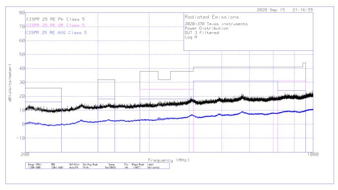
Figure 6-5. Radiated Emissions - Logarithmic Horizontal Antenna 200 MHz to 1000 MHz
