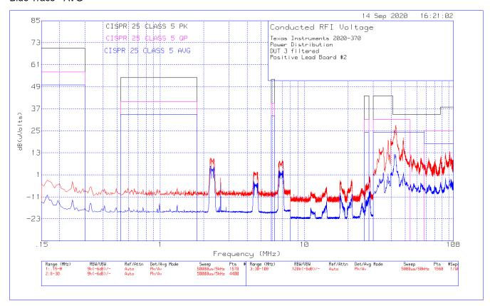
Figure 6-1. Conducted Emissions 0.15 MHz to 108 MHz
