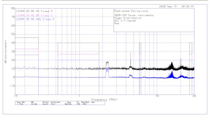
Figure 6-2. Radiated Emissions - Rod Antenna 0.15 MHz to 30 MHz
