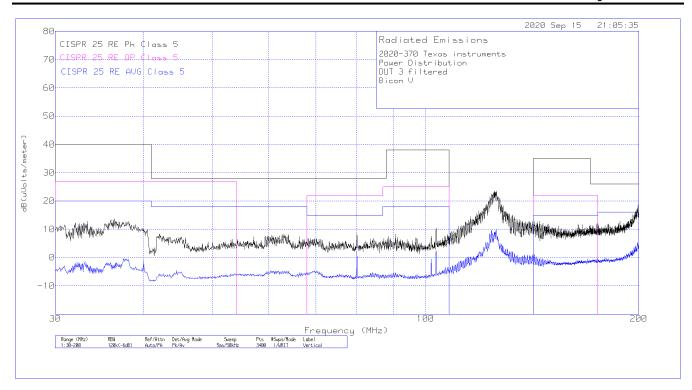
Figure 6-4. Radiated Emissions - Bicon Vertical Antenna 30 MHz to 200 MHz
