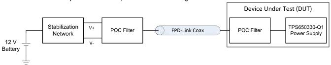
Figure 3-1. CISPR-25 EMC Test Setup
