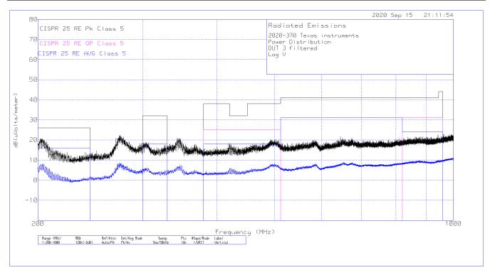
Figure 6-6. Radiated Emissions - Logarithmic Vertical Antenna 200 MHz to 1000 MHz
