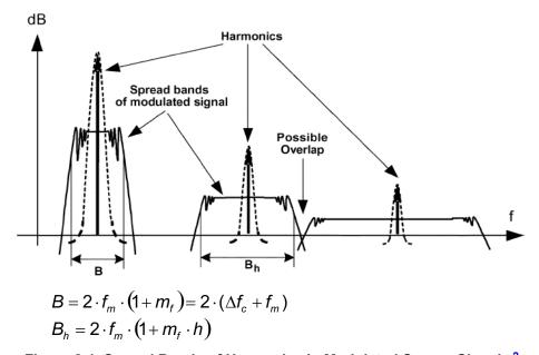
Figure 2-1. Spread Bands of Harmonics in Modulated Square Signals <sup>2</sup>
