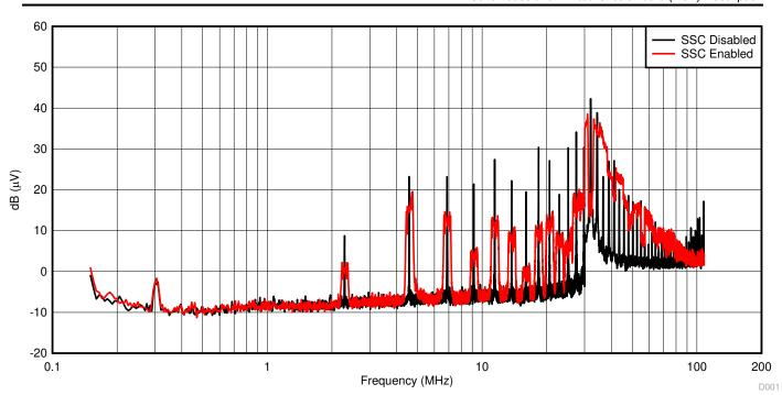
Figure 2-2. TPS650330-Q1 SSC Conducted Emission Comparison
