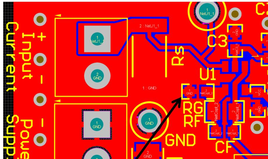
Gain setting resistor moved close to GND of shunt resistor
