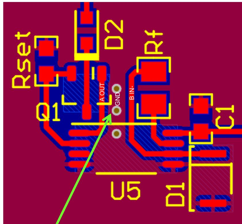
Add GND pour with vias between CH A Output and CH B IN-
