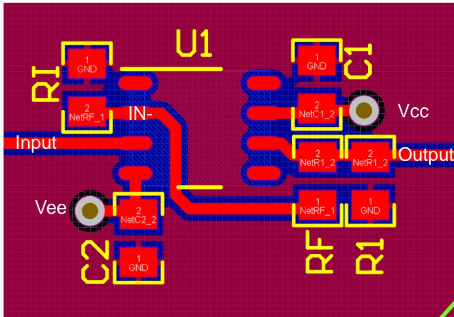
Inverting input traces kept as small as possible
