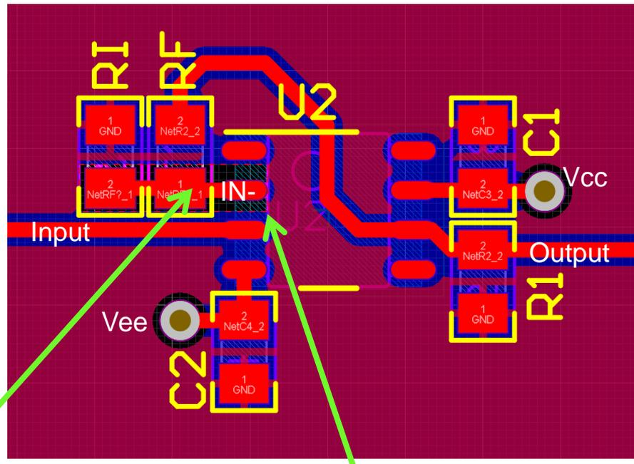
Ground plane removed from inverting input node to reduce stray capacitance
